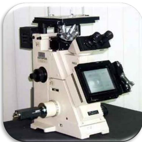
*Figure 16. (Metallograph/ Microscope.)*
