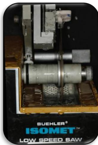
Figure 12. (Low-speed diamond saw with diamond wafering blade.)
