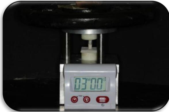
*Figure 10. (Cemented coping-die assembly placed under static load of 49 N.)*
