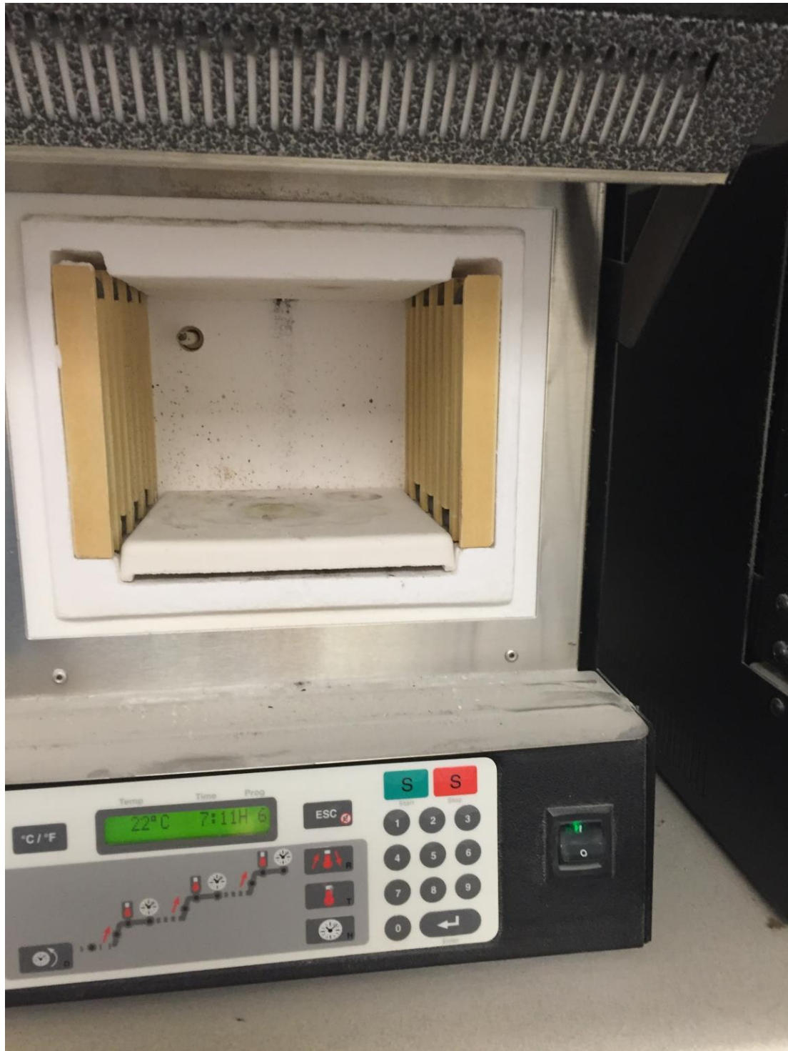
Figure 2. Heating Chamber of Neytech Vulcan Multi-stage Programmable Furnace
