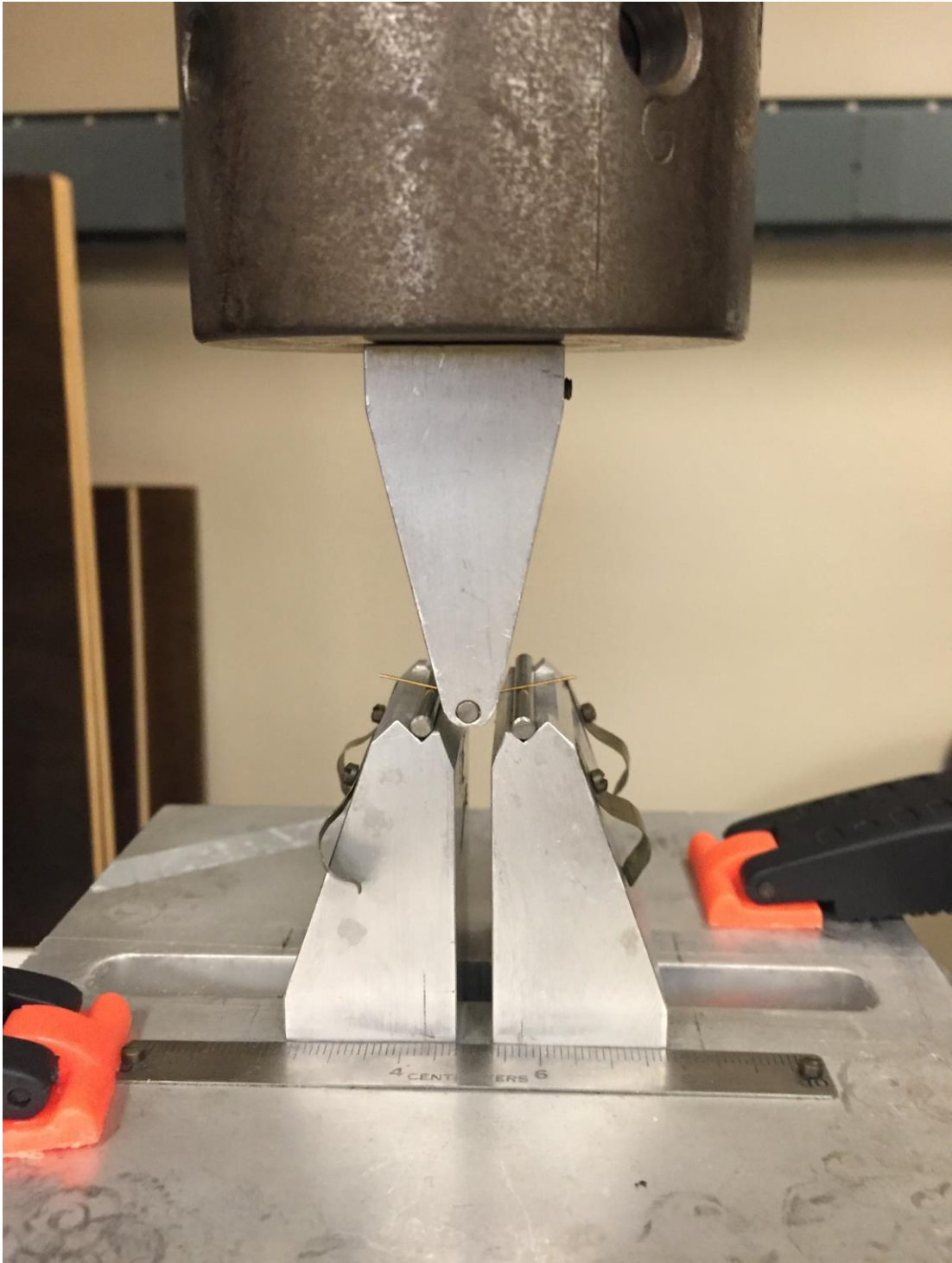
Figure 4. Instron Universal Testing Machine Performing Three-Point Bend Test
