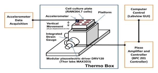
**Mechanical Vibration Set-up Diagram**
