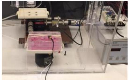
**Figure 7**: Enclosed thermal box at 37<sup>o</sup>C. Platform delivering vibration to plate of cells. Accelerometer attached on top of plate.
