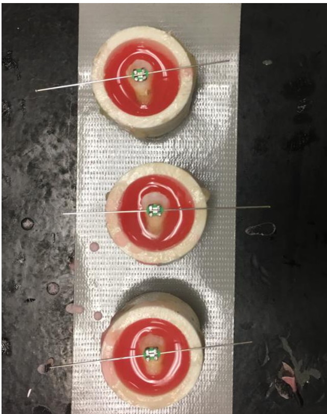
Figure 7. Three bonded teeth in cold-cure acrylic as the acrylic set up
