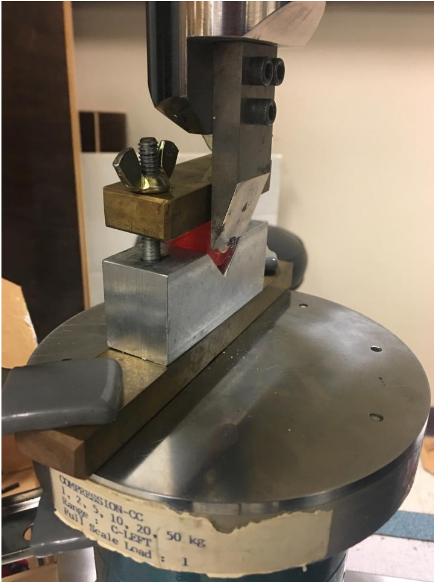
Figure 10. Each tooth secured in the universal testing machine to test the shear bond strength
