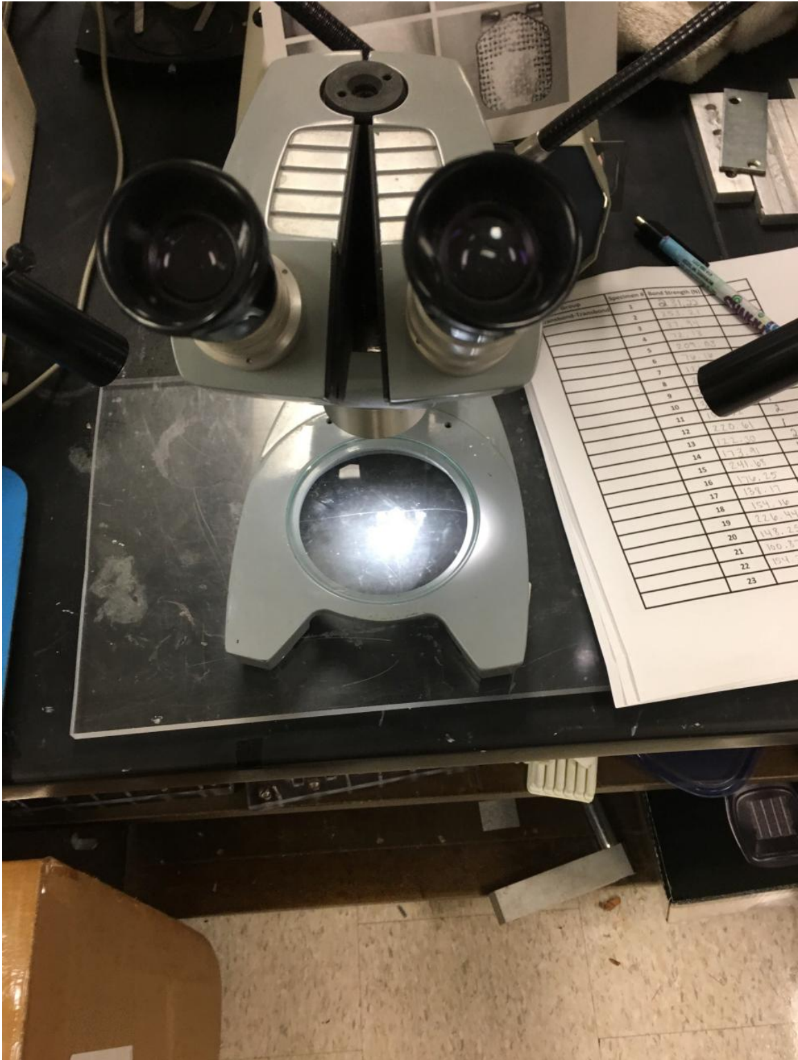
Figure 12. Microscope used to measure the ARI
