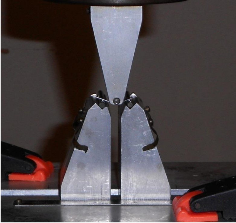
Figure 3. Three-point bending test in progress.
