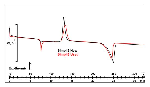
Figure 9: Comparison between as-received and used Simpli5 samples
