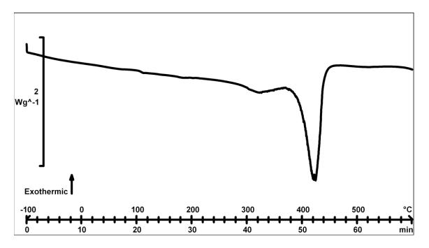
**Figure 6:** As-received Invisalign, wide temperature scan. Peaks are much more subtle, the small inflection around 100°C represents the glass transition phase. The large endothermic peak near 420°C represents decomposition of the material.
