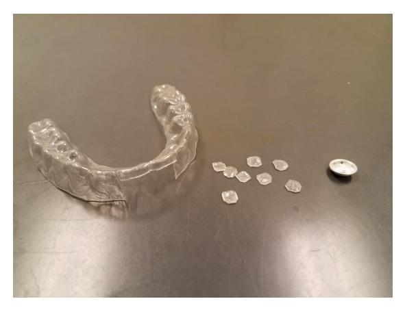
**Figure 3:** As-received Simpli5 aligner with a section removed for sampling, cut samples, and a prepared and sealed aluminum crucible ready for testing
