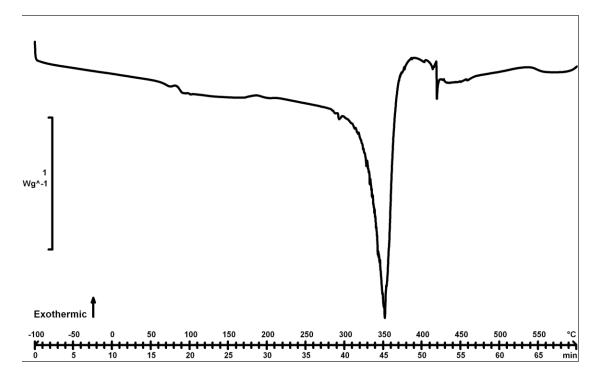
**Figure 7:** As-received ClearCorrect, wide temperature scan. The sigmoidal event around 80°C represents the glass transition phase. The large endothermic peak near 350°C represents decomposition of the material.
