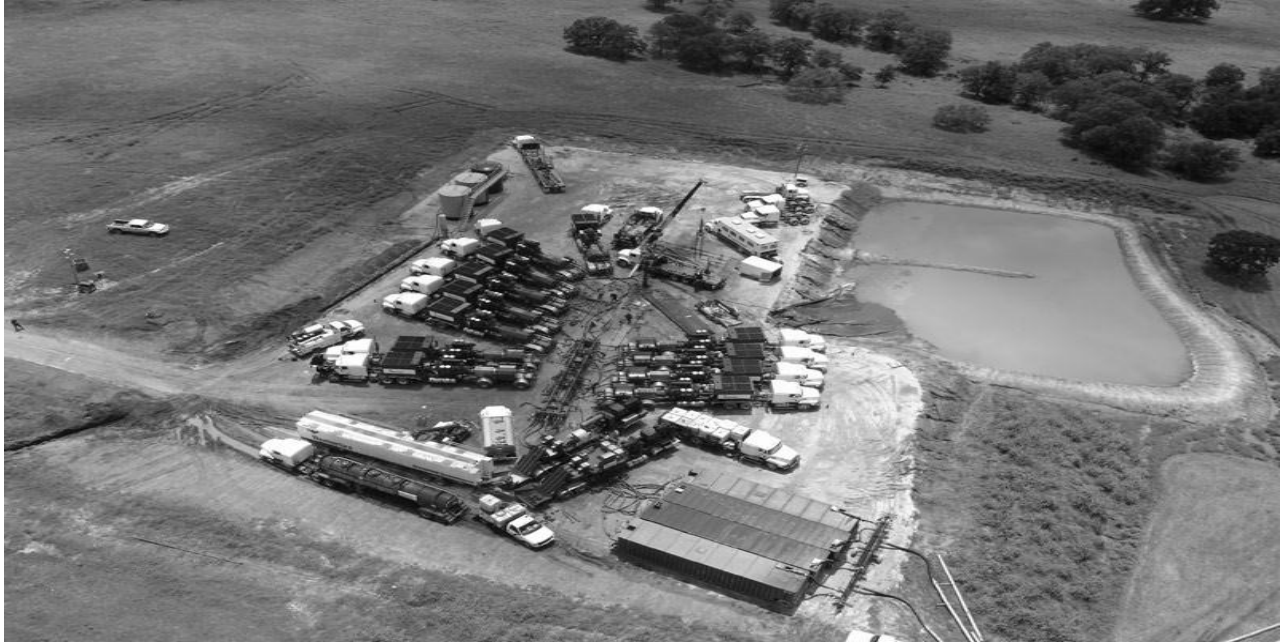
Figure 1.1: A drilling site where hydraulic fracturing is taking place. A reserve pit the size of a swimming pool is seen adjacent to the drilling rig. The trucks pump in millions of gallons of fracturing fluid under high rate to crack the dense organic gas-bearing shale rock several thousands of feet below. Drilling mud is stored in the reserve pit. If the reserve pit overflows due to excessive rainfall or one of its earthen walls collapses, there can be severe environmental consequences. (Photo courtesy: Tom Hayes of Gas Technology Institute)
