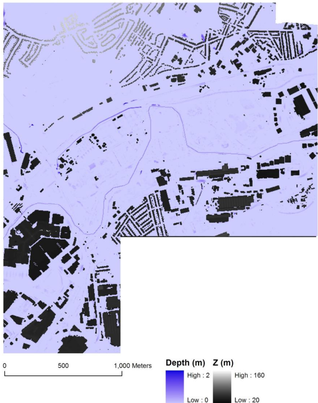
Figure 6.6 Flood inundation extent taken from 80000 seconds (~22 hours) into simulation 3, populated with initial depth mask corrected for buildings and unknown areas.
