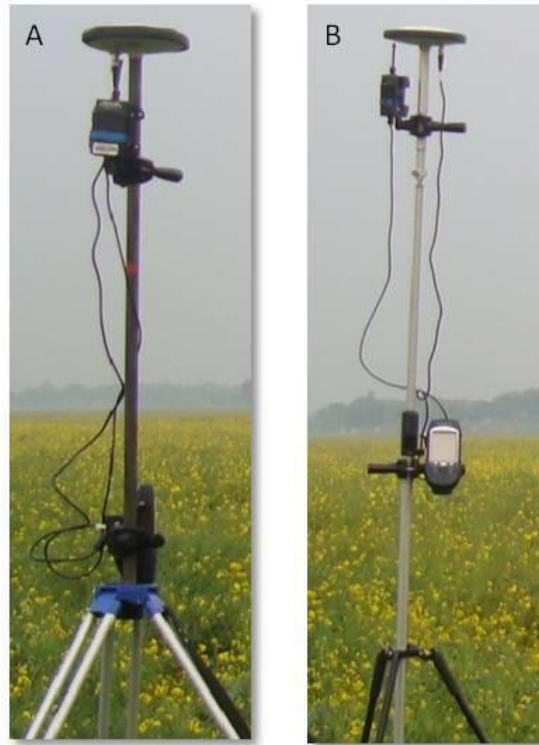
Figure 5.4: ProMark3-RTK dGPS equipment - Base station (A) and Rover (B).
