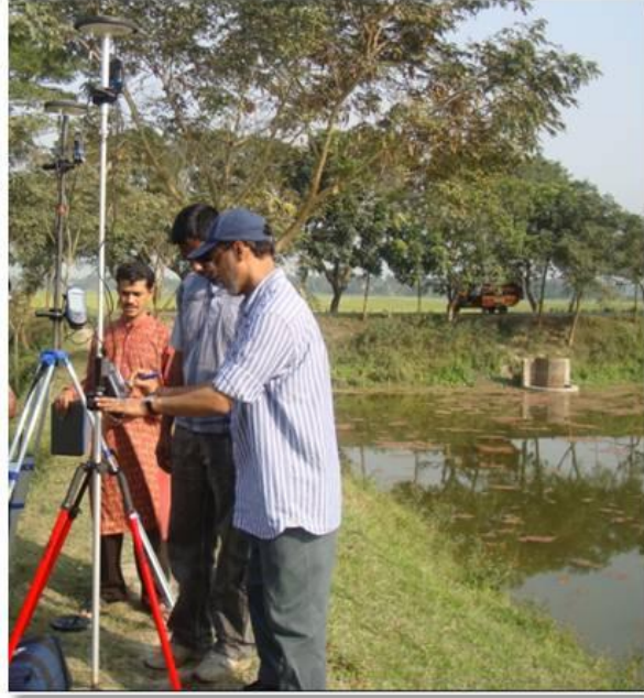
Figure 5.5: Setting up the ProMark3 equipment (base and rover) during fieldwork in Bangladesh.
