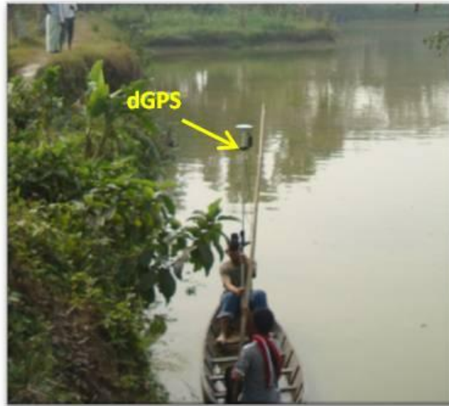
Figure 5.3: Using a small local boat carrying dGPS-Rover equipment to avoid access limitation and steep areas.
