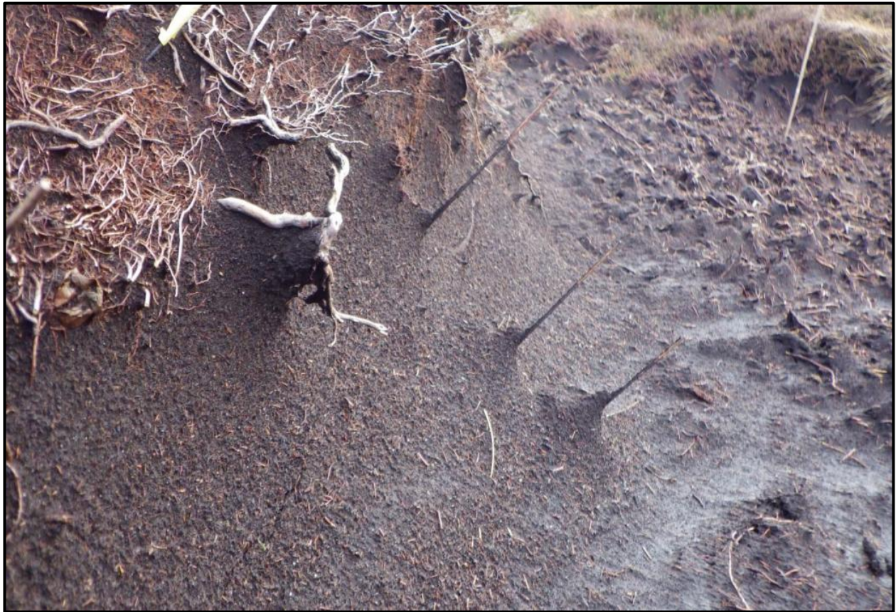
Figure 8.2 – Pedestals observed at the base of some erosion pins during field visits. These could lead to false negative values of change in pin exposure.
