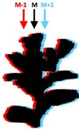
Figure 4.40 Schematic of pressure values extracted from one cell immediately upstream ( M-1 ) and downstream ( M+1 ) of the plant blockage ( M ), used in the calculation of drag forces.
