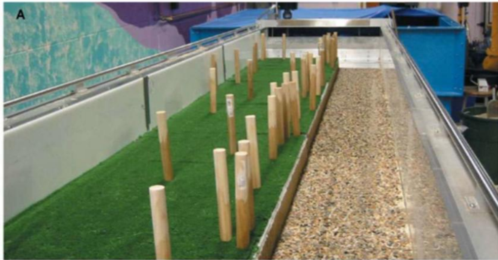
Figure 2.18 Example of dowel rods used to represent floodplain vegetation from McBride et al. (2007).
