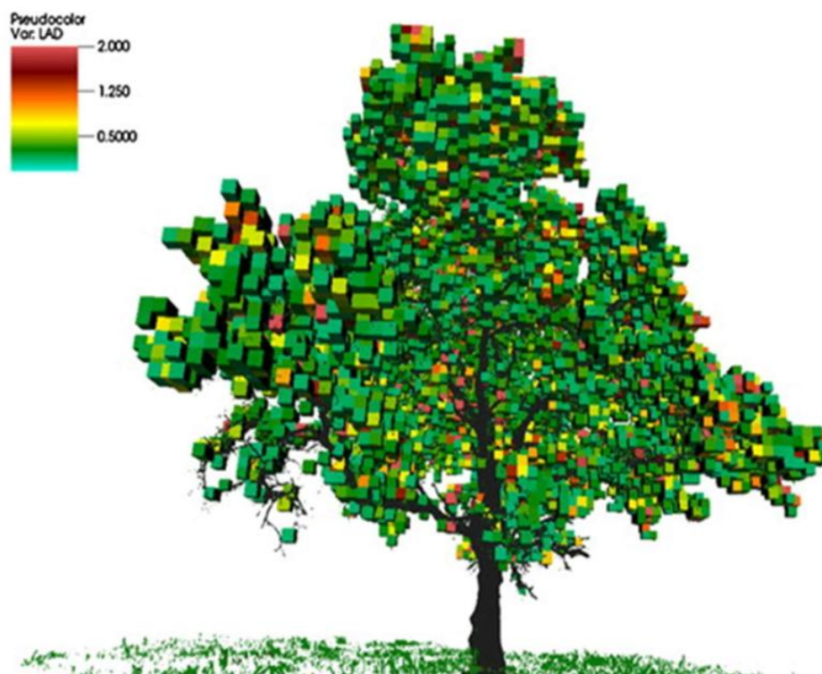
Figure 3.11 Application of a voxel based approach to TLS data, displaying the spatially explicit measure of leaf area distribution. Colours indicate leaf area estimates per voxel, from red (highest density) to green (lowest density). A 0.15 m voxel size is used to describe the distribution of leaf area, from Béland et al. (2014a).
