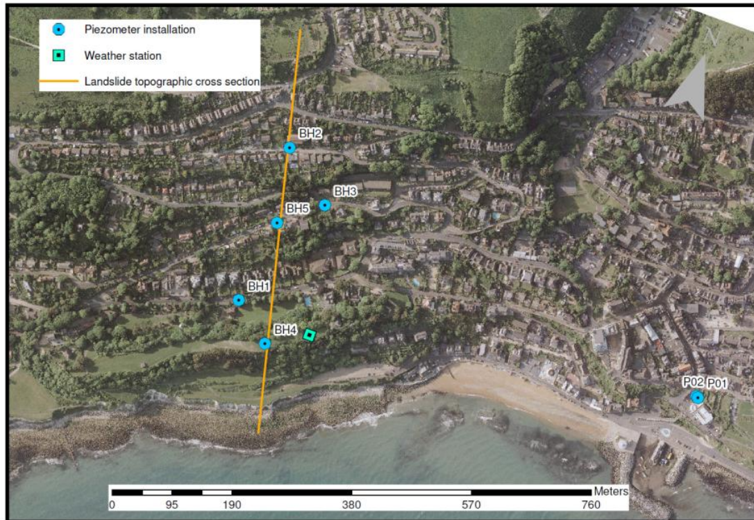
Figure 5.24 Piezometer and weather station locations, Ventnor Town
