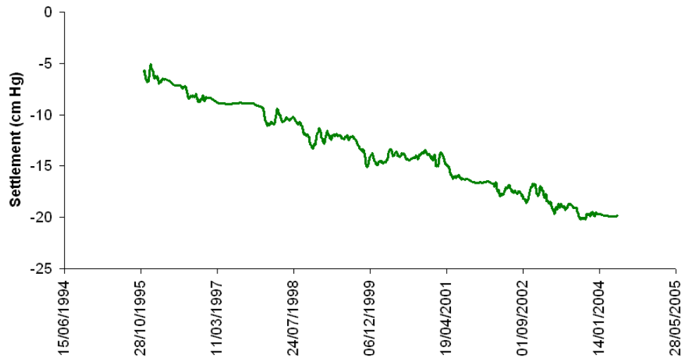
Figure 5.18 Running mean settlement measured at SC06, Bath Road (1995-2004)
