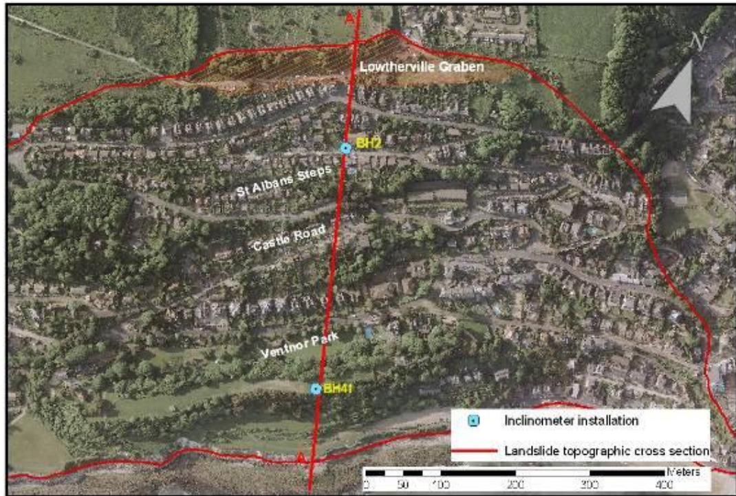
Figure 5.2 Location of Inclinometers within the Ventnor landslide complex
