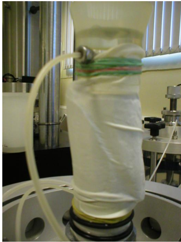
Plate 6.1 Classic Brittle failure through shear surface development sample ICU1
