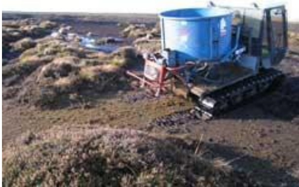
Figure 2.2: The machine used to spread the heather brush across the bare peat surface. For scale the machine is approximately 1.5 m wide. Source: Peatscapes
