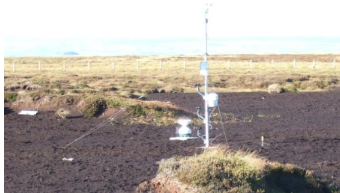
Figure 3.12: The Automatic Weather Station measuring wind speed at 4 heights, wind direction, air temperature, soil tension and temperature and precipitation. One of the erosion pin and sediment trough sites is visible in the background.
