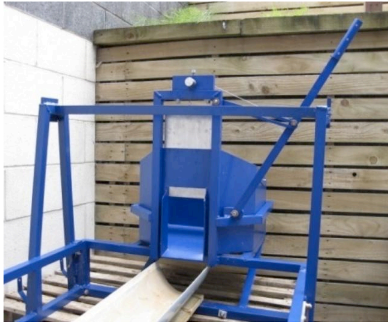
Figure 3.7: Photograph of the mixture container and release gate attached to the head of the large outdoor flume.
