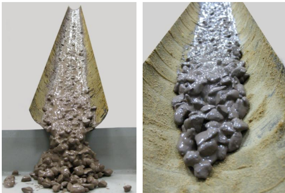
Figure 3.3: Photographs of typical debris flow mixtures used in the small laboratory flume. The roughened channel and variations in particle size are visible.
