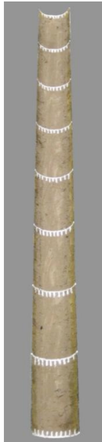
Figure 3.2: Photograph of the small laboratory flume channel with reference markings; horizontal lines every 0.25 m along the flume length denoting every 0.01 m of the channel width.
