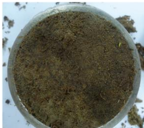
Figure 3.14 Example of a full sample collected within the oedometer ring.
