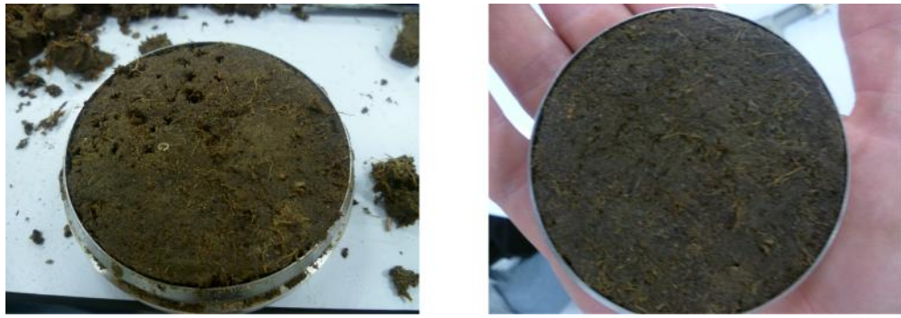
Figure 3.18: Root removal and then subsequent 'repair' is shown for oedometer samples.
