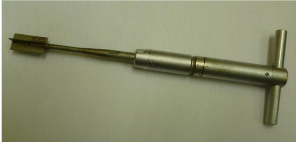
Figure 3.12 Geonor H-60 hand-held shear vane tester. Testing was carried out by placing the bladed vane (left) into the ground, turning the handle and upon the sediment failure the torque measurement was recorded.
