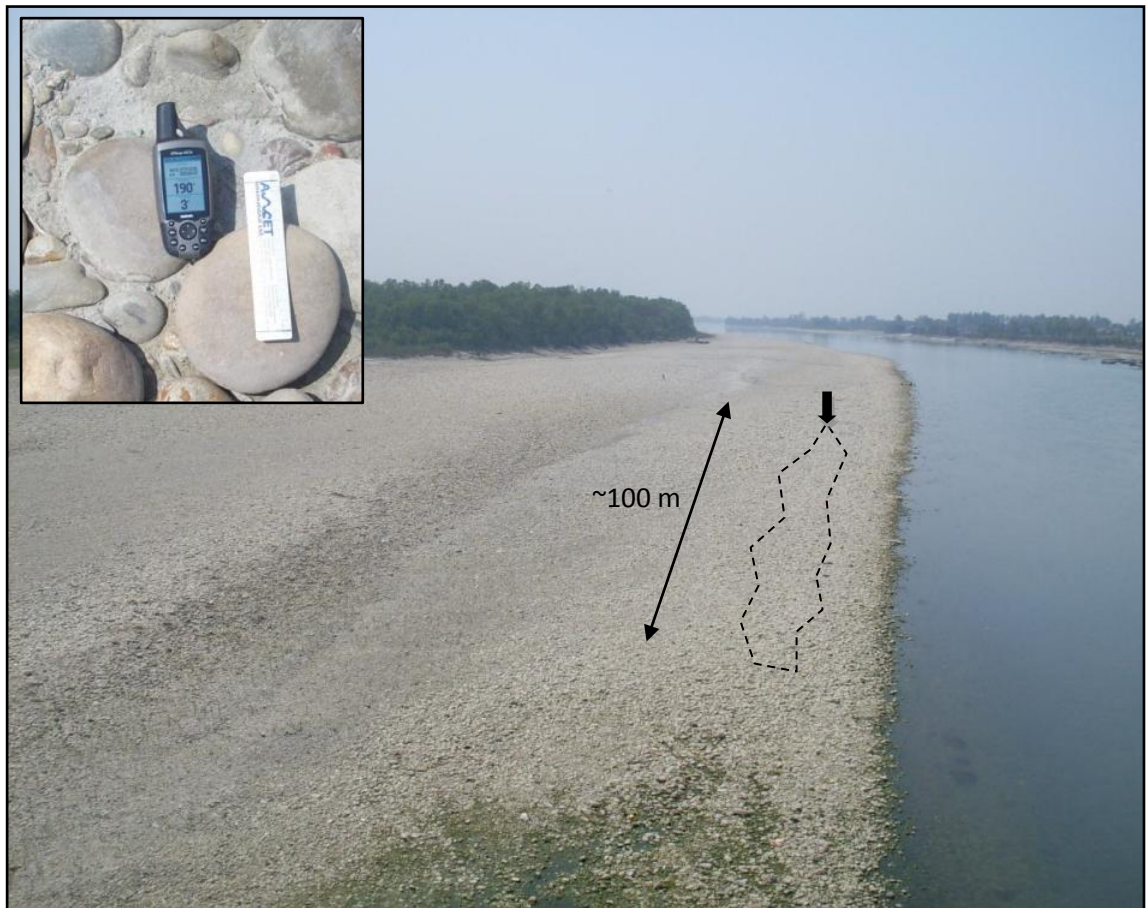
Figure 3.4. Typical transect path as indicated by the dashed line. The first photo as indicated by the arrow would contain both the GPS and 150 mm scale as shown in the top left corner. Depending on the size of the bar and quality of the exposure, samples may contain up to 100 photos each taken a few steps apart. For reference, this image is facing downstream.
