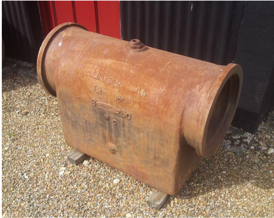
Figure 12 - Photograph of a water trap used for separating water from town gas (Fakenham Gas Museum, 2014)
