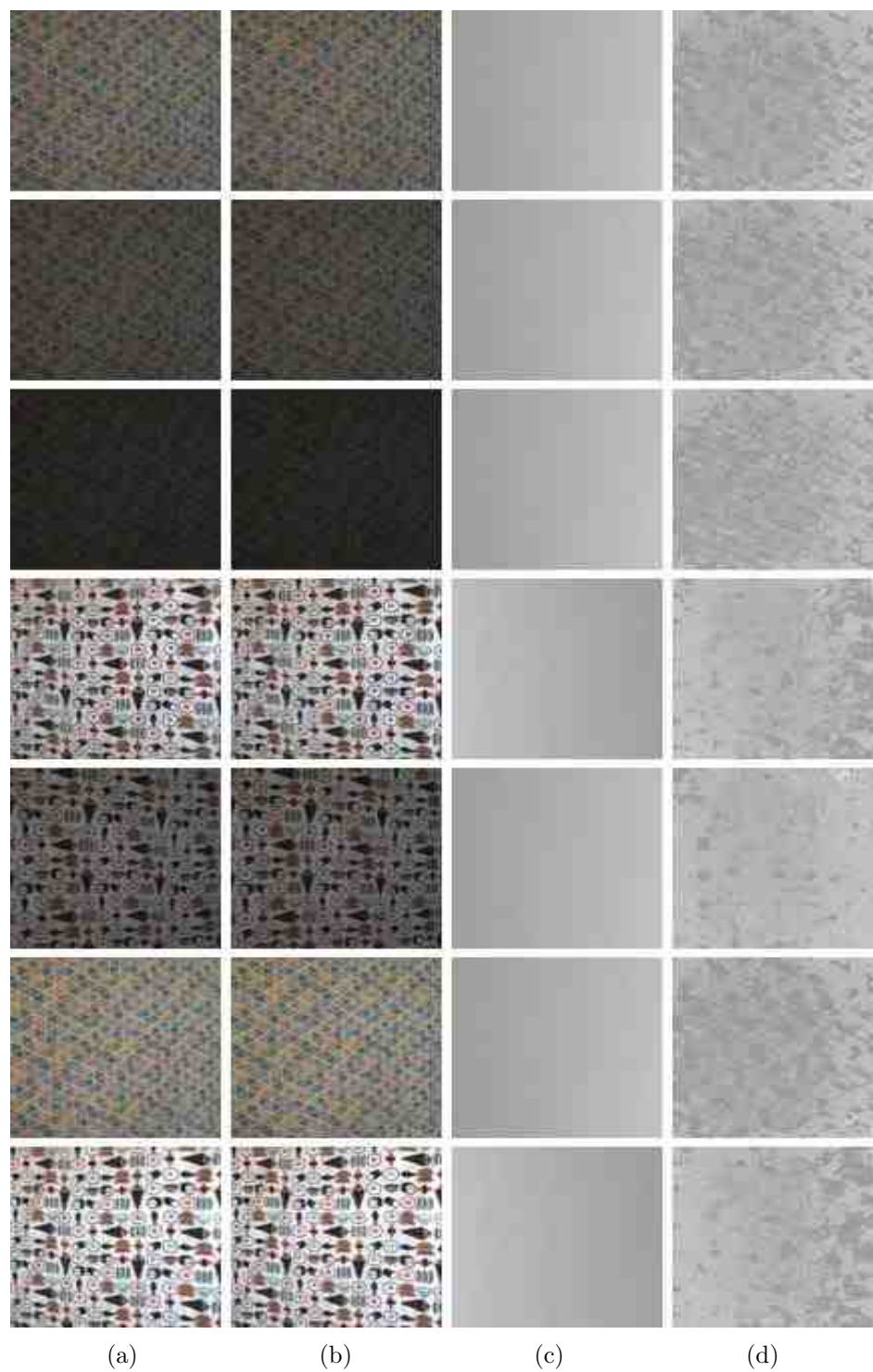
Fig. F.1. Performance Results for the DfD-Net on the Real World Dataset - Part 1. (a) In-focus Image, (b) Out-of-focus Image, (c) Ground Truth Depth Map and (d) DfD-Net Computed Depth Map.
