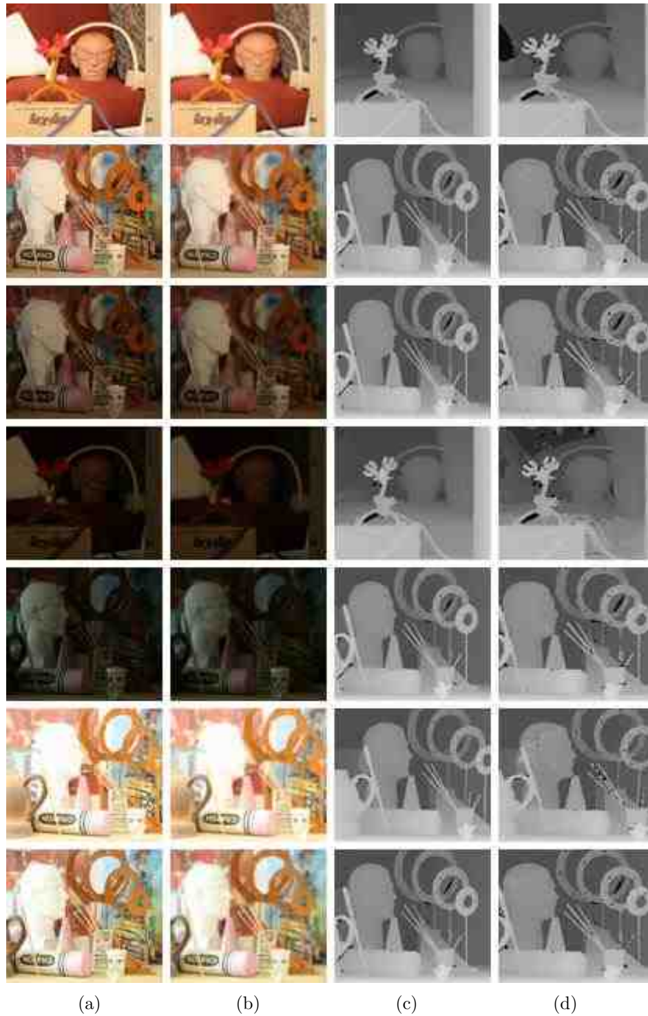
Fig. C.6. PSO Performance Results for the Middlebury College Dataset - Part 6. (a) In-focus Image, (b) Out-of-focus Image, (c) Ground Truth Depth Map and (d) DfD-Net Computed Depth Map.
