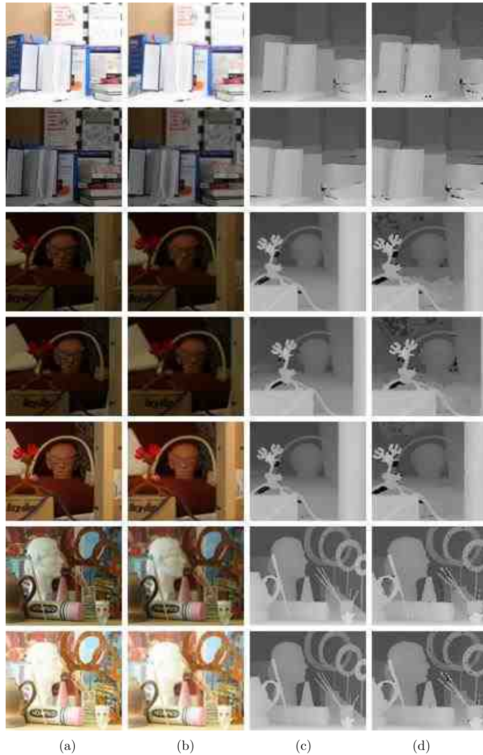
Fig. C.4. PSO Performance Results for the Middlebury College Dataset - Part 4. (a) In-focus Image, (b) Out-of-focus Image, (c) Ground Truth Depth Map and (d) DfD-Net Computed Depth Map.
