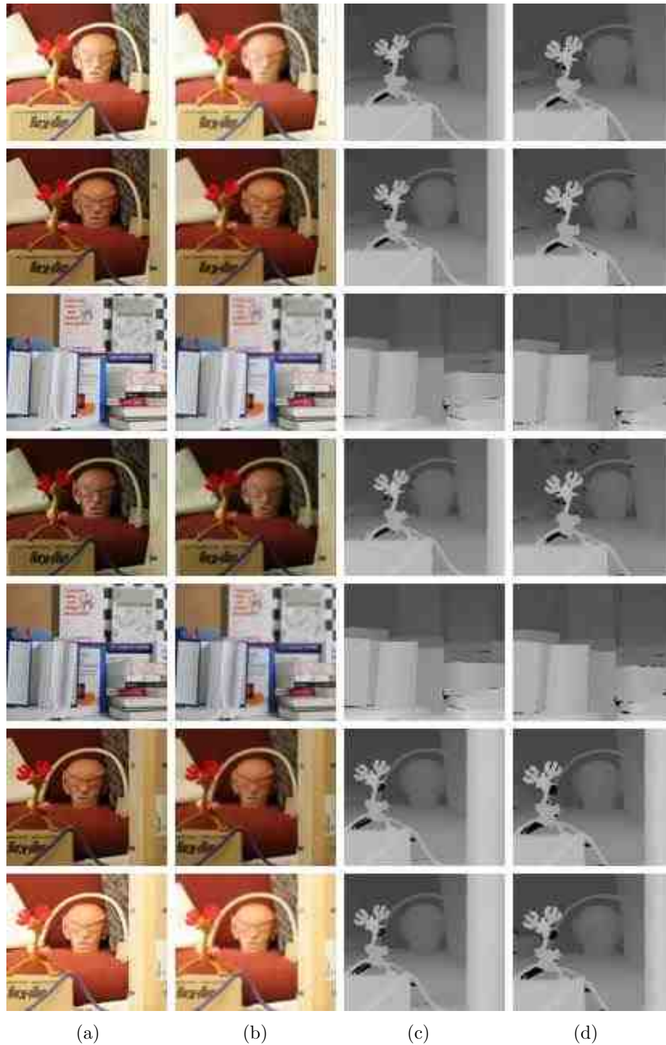
Fig. D.2. Filter Reduction Performance Results for the Middlebury College Dataset - Part 1. (a) In-focus Image, (b) Out-of-focus Image, (c) Ground Truth Depth Map and (d) DfD-Net Computed Depth Map.
