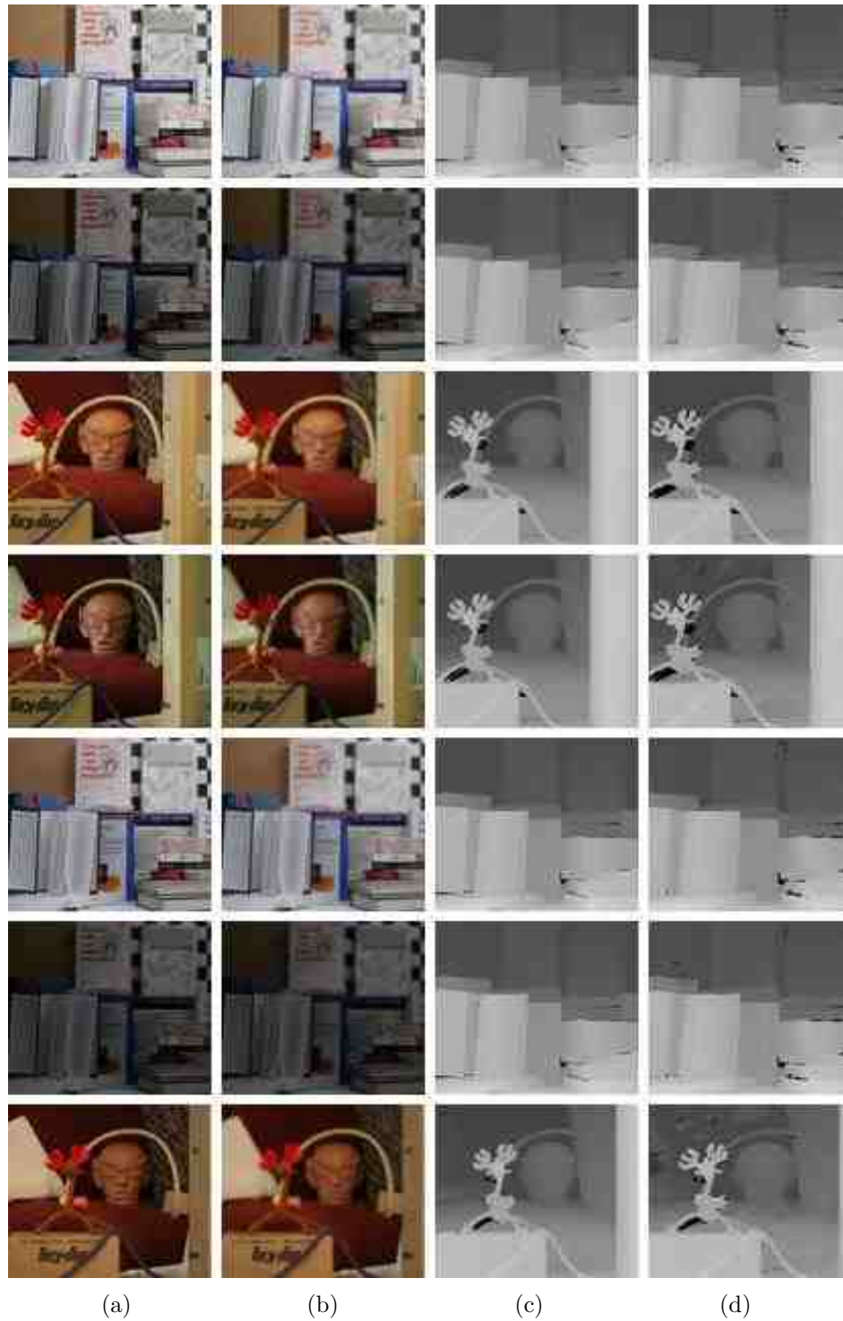
Fig. C.3. PSO Performance Results for the Middlebury College Dataset - Part 3. (a) In-focus Image, (b) Out-of-focus Image, (c) Ground Truth Depth Map and (d) DfD-Net Computed Depth Map.
