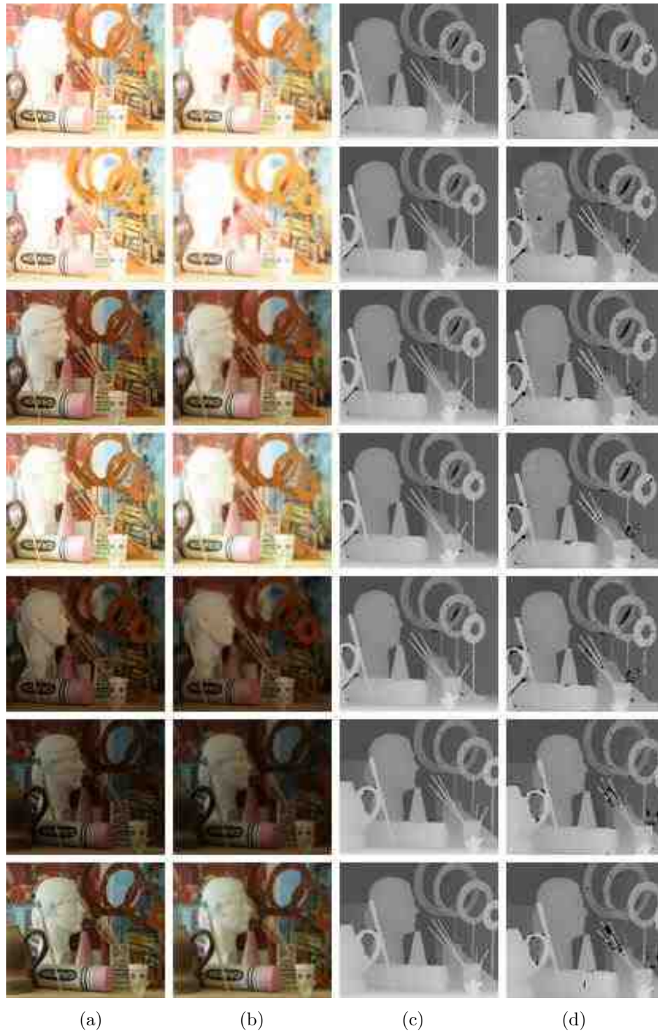
Fig. D.8. Filter Reduction Performance Results for the Middlebury College Dataset - Part 7. (a) In-focus Image, (b) Out-of-focus Image, (c) Ground Truth Depth Map and (d) DfD-Net Computed Depth Map.
