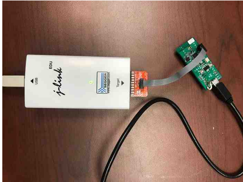
Fig. 6.2. Bootloading with JLINK Debugger
