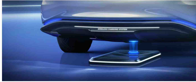
Fig. 2.7. Example of a potential inductive WPT solution for cars [18]
