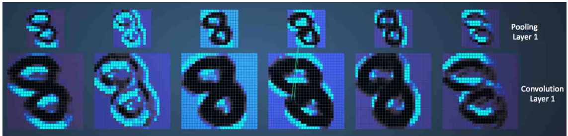
Fig. 2.9. Visualizing the Pooling Operation.
