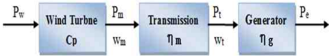
Fig. 3.1. Energy Conversion Chart of wind generation system.
