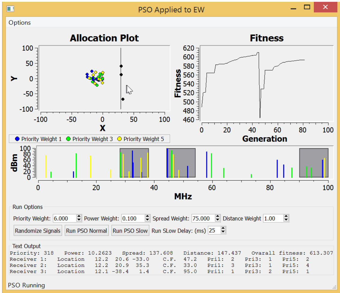
Fig. 3.2. Click event from user triggers a change in Keep Away Boundary. A downward spike in fitness occurs as solution fitness is penalized for receivers being outside of bounds.
