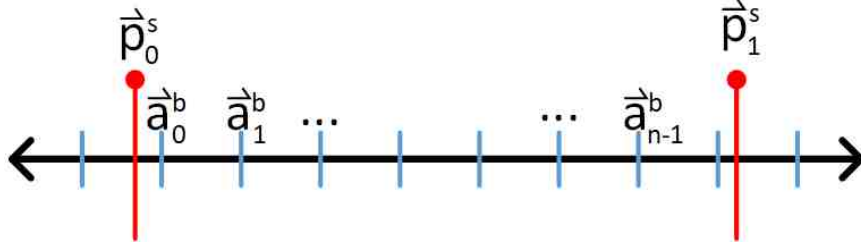
Fig. 2.1. The data rate of the accelerometer is faster than, and unsynchronized with the frame rate of the Camera being used for SLAM.
