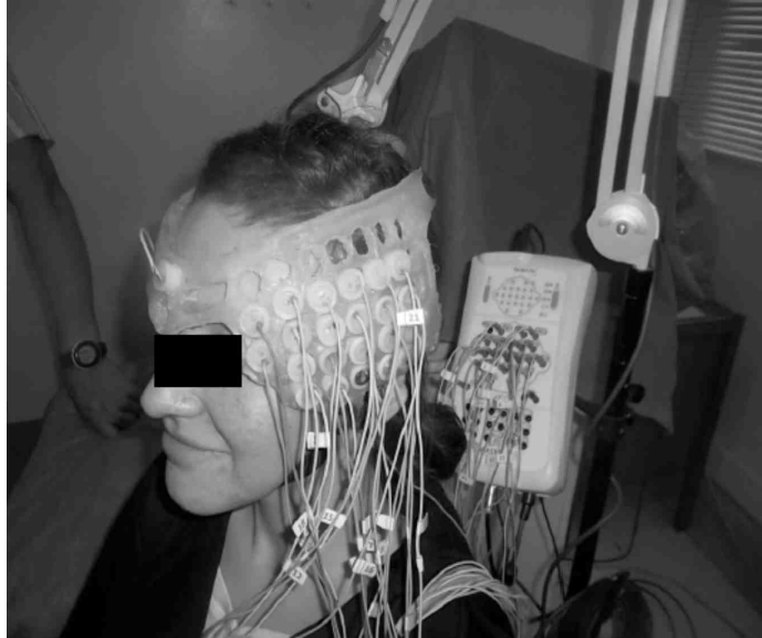
Fig. 4.2: Subject wearing the silicon EEG neuro-headset with 21 electrodes on the left hemisphere plus one frontal reference electrode.
