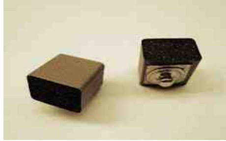
Fig. 2.6: Dry foam electrode fabricated by electrically conductive polymer.
