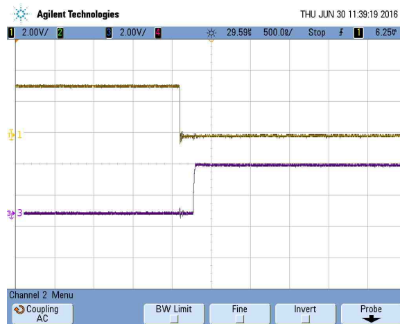
Fig. B.2. Dead time generated between the ports RB5 and RB7
