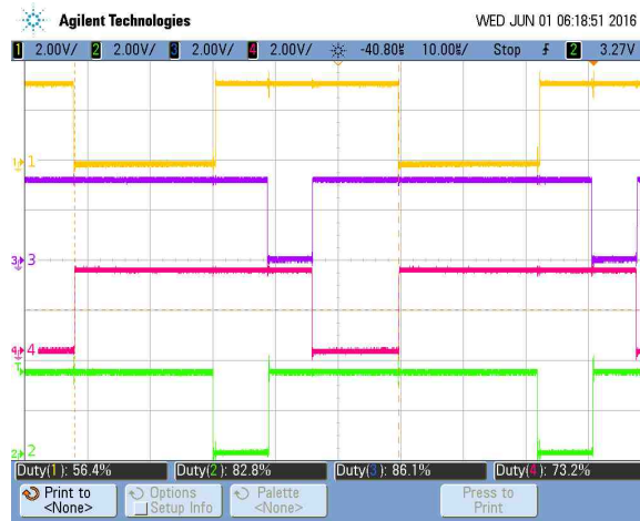
Fig. B.1. PWM signals generated from the DSPIC 33F64FJMC802
