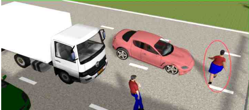
(a) Vehicle started applying break using V2V-AEB system
