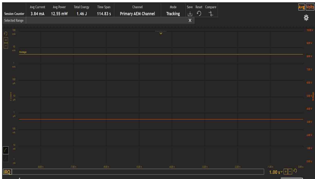
Fig. 7.9. The MPU6050 Active Mode Power Consumption
