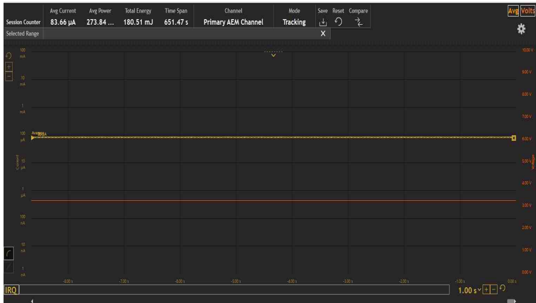
Fig. 7.8. The ADXL345 and MCU Deep Sleep Mode Power Consumption
