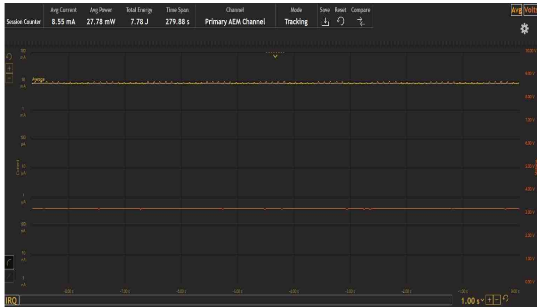
Fig. 7.11. The BLE Connected Mode Power Consumption
