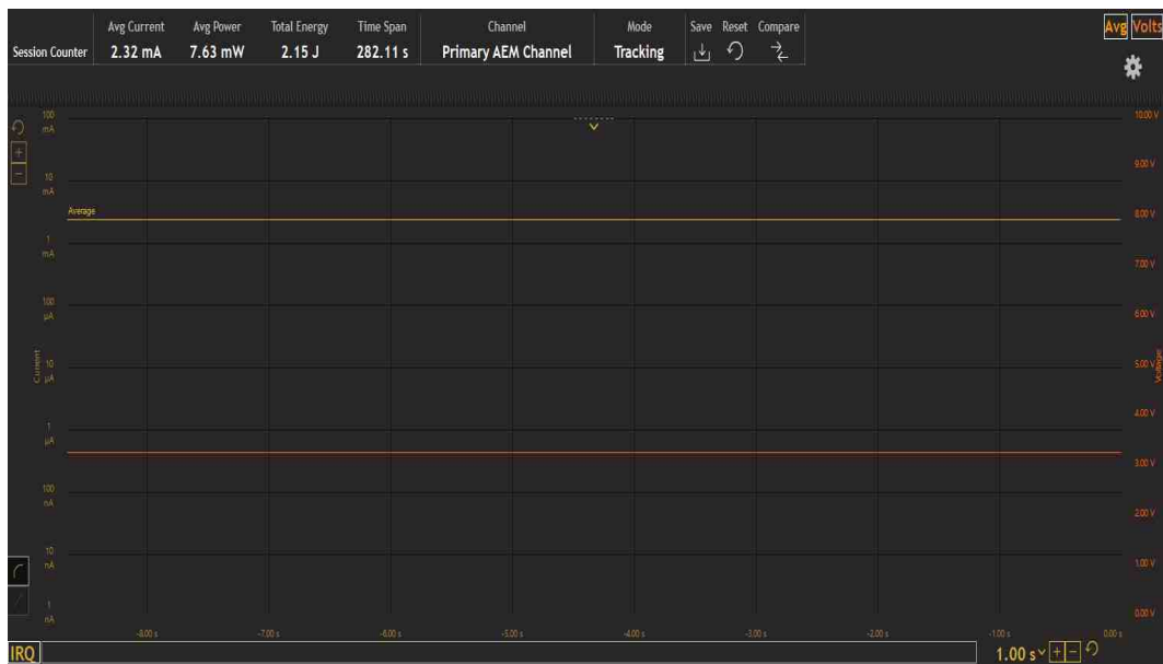
Fig. 7.7. The MCU Active Power Consumption
