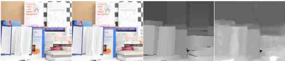
Fig. 4.62.: Second best performance in the Middlebury dataset. In-focus image, out of focus image, ground truth, and generated depth map
