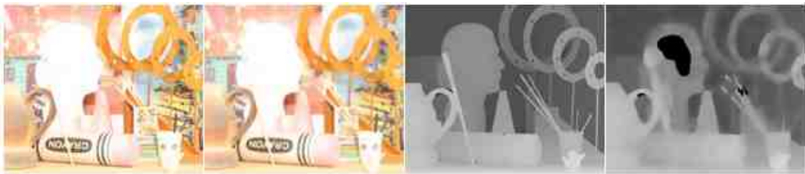
Fig. 4.24.: Second worst performance in the Middlebury dataset. In-focus image, out of focus image, ground truth, and generated depth map
