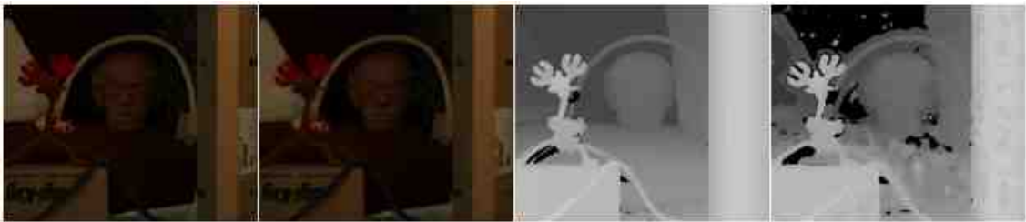
Fig. 4.30.: Worst performance in the Middlebury dataset. In-focus image, out of focus image, ground truth, and generated depth map
