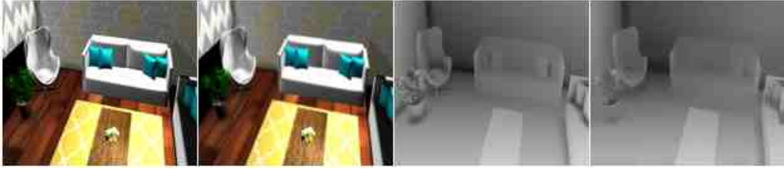
Fig. 4.3.: In-focus image, blurred image, ground truth and estimated depth map
