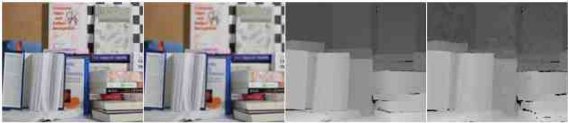
Fig. 4.29.: Second best performance in the Middlebury dataset. In-focus image, out of focus image, ground truth, and generated depth map
