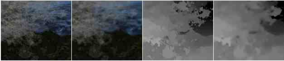
Fig. 4.19.: Worst performance in the Maya dataset. In-focus image, out of focus image, ground truth, and generated depth map
