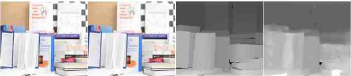
Fig. 4.55.: Second best performance in the Middlebury dataset. In-focus image, out of focus image, ground truth, and generated depth map
