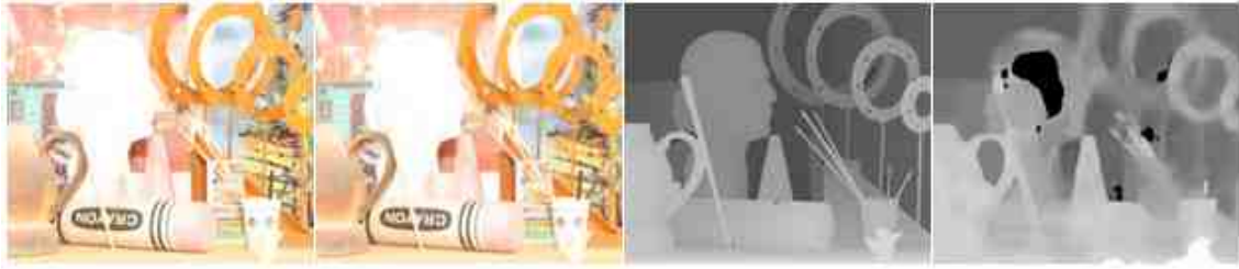
Fig. 4.64.: Second worst performance in the Middlebury dataset. In-focus image, out of focus image, ground truth, and generated depth map
