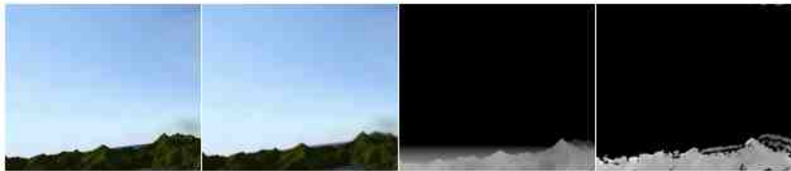
Fig. 4.65.: Best performance in the Maya dataset. In-focus image, out of focus image, ground truth, and generated depth map
