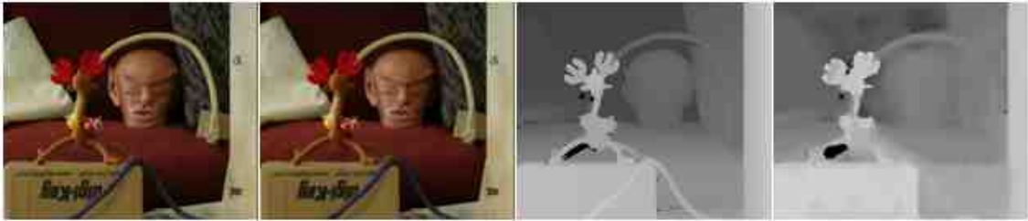
Fig. 4.61.: Best performance in the Middlebury dataset. In focus image, out of focus image, ground truth, and generated depth map
