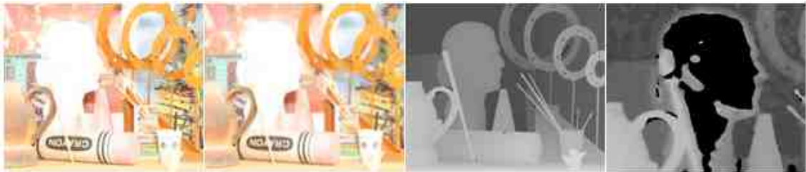
Fig. 4.45.: Worst performance in the Middlebury dataset. In-focus image, out of focus image, ground truth, and generated depth map
