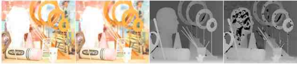
Fig. 4.31.: Second worst performance in the Middlebury dataset. In-focus image, out of focus image, ground truth, and generated depth map
