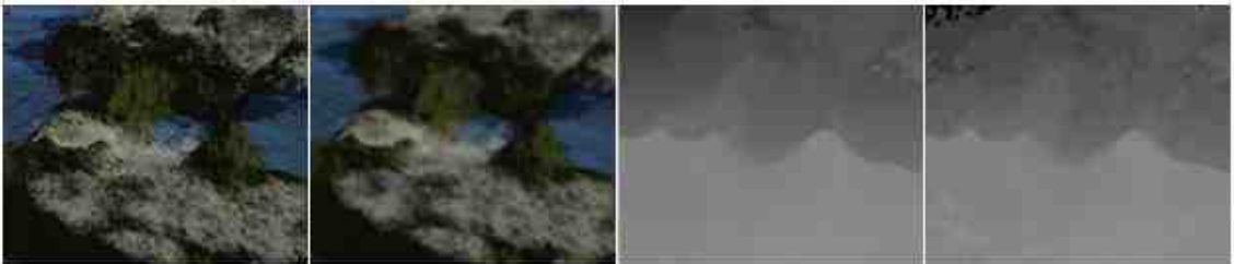
Fig. 4.33.: Second best performance in the Maya dataset. In-focus image, out of focus image, ground truth, and generated depth map
