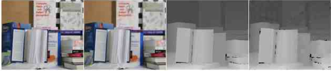
Fig. 4.28.: Best performance in the Middlebury dataset. In-focus image, out of focus image, ground truth, and generated depth map
