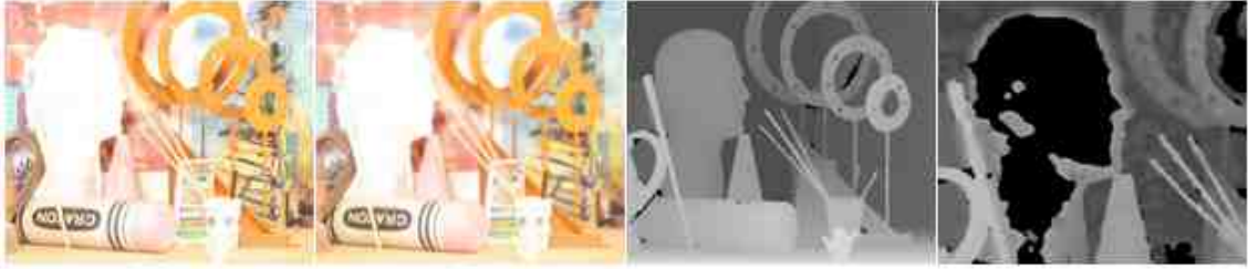
Fig. 4.46.: Second worst performance in the Middlebury dataset. In-focus image, out of focus image, ground truth, and generated depth map
