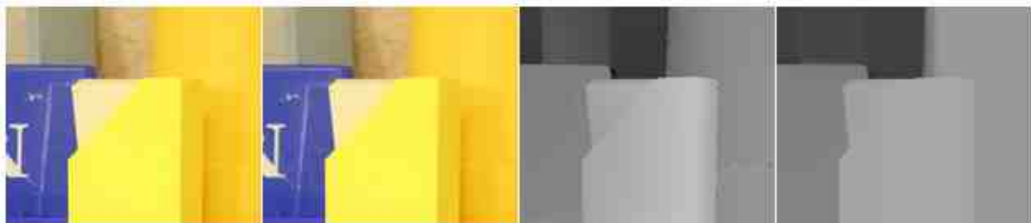
Fig. 4.1.: In-focus image, blurred image, ground truth and estimated depth map
