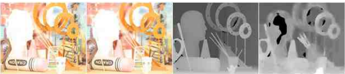
Fig. 4.63.: Worst performance in the Middlebury dataset. In-focus image, out of focus image, ground truth, and generated depth map
