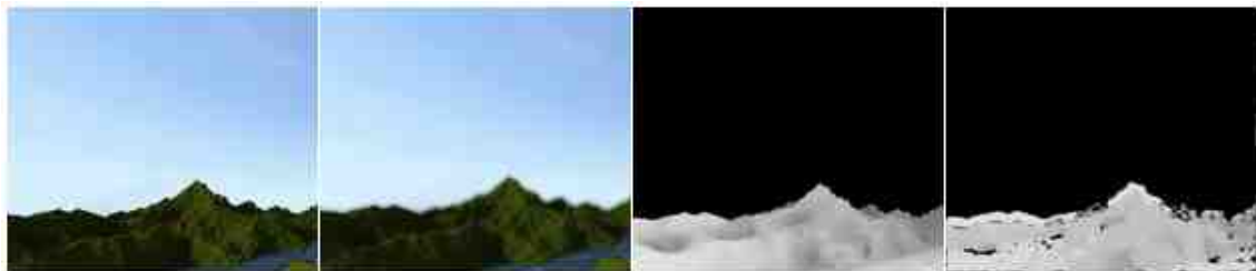
Fig. 4.66.: Second best performance in the Maya dataset. In-focus image, out of focus image, ground truth, and generated depth map
