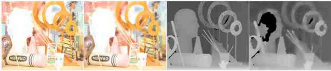
Fig. 4.23.: Worst performance in the Middlebury dataset. In-focus image, out of focus image, ground truth, and generated depth map
