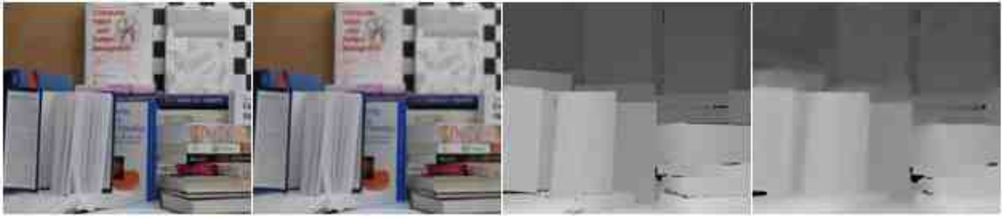
Fig. 4.22.: Second best performance in the Middlebury dataset. In-focus image, out of focus image, ground truth, and generated depth map
