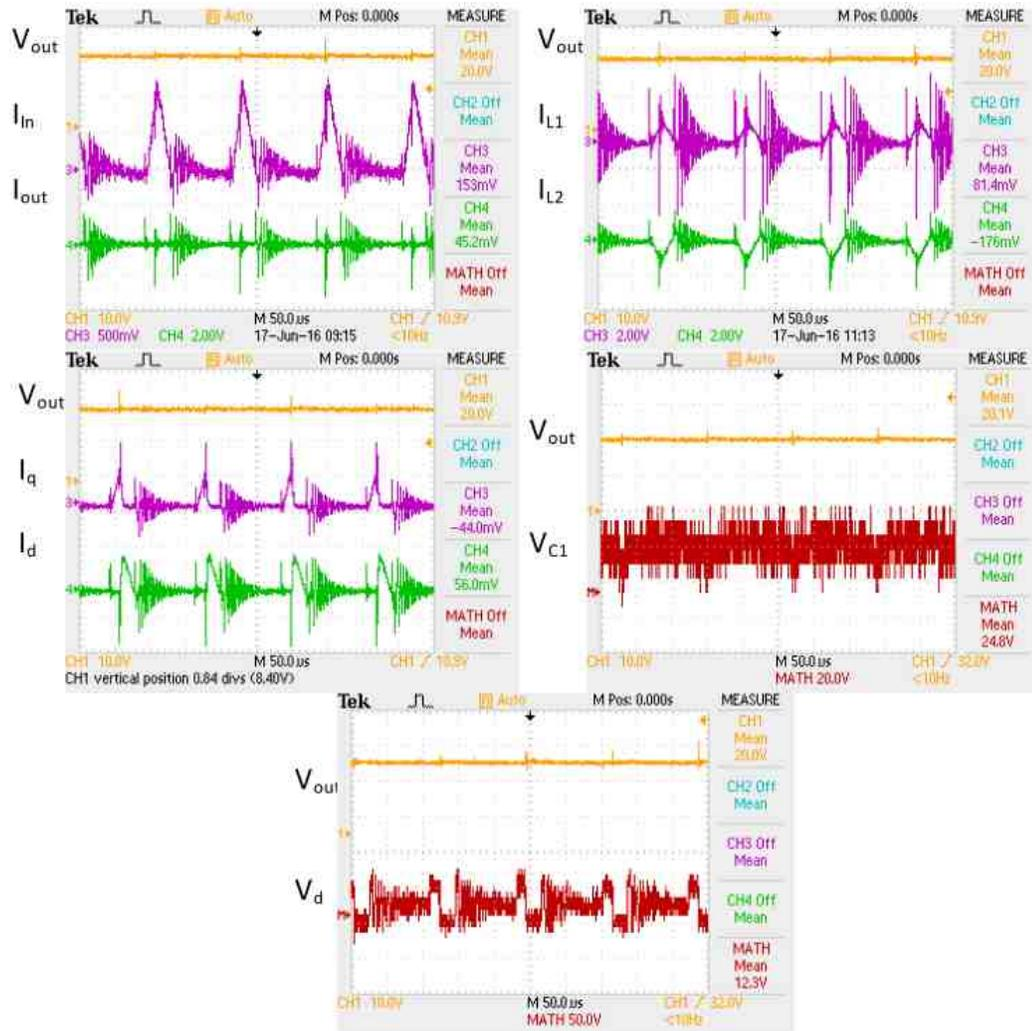
Fig. 4.5. Output Voltage  $V_o$ , Source Current  $I_g$ , Output Current  $I_o$ , Inductors Current  $I_{L1}$  &  $I_{L2}$ , Diode Current  $I_d$ , Transistor Current  $I_q$ , Capacitor  $C_1$  Voltage  $V_{C1}$ , and Diode Voltage  $V_d$  for positive buck mode.
