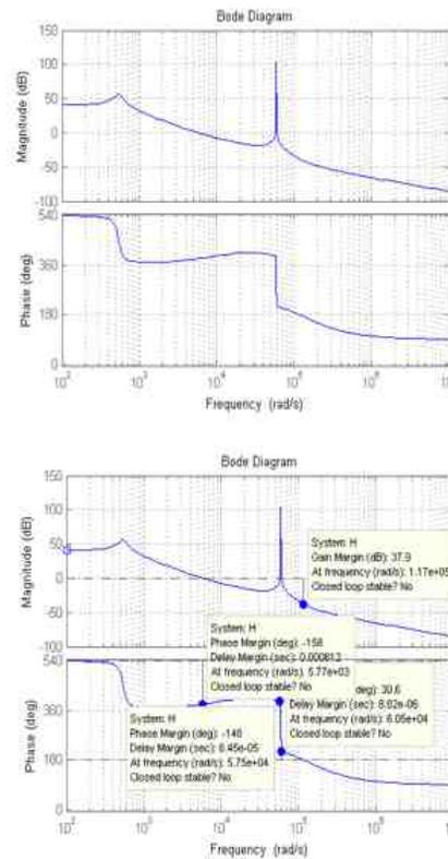
Fig. 3.9. Bode Plots for Negative Output Voltage
