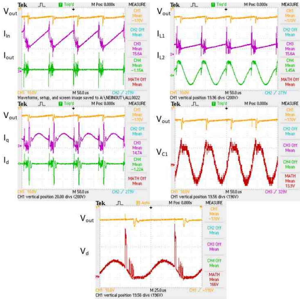
Fig. 4.6. Output Voltage  $V_o$ , Source Current  $I_q$ , Output Current  $I_o$ , Inductors Current  $I_{L1}$  &  $I_{L2}$ , Diode Current  $I_d$ , Transistor Current  $I_q$ , Capacitor  $C_1$  Voltage  $V_{C1}$ , and Diode Voltage  $V_d$  for negative boost mode (-170V).
