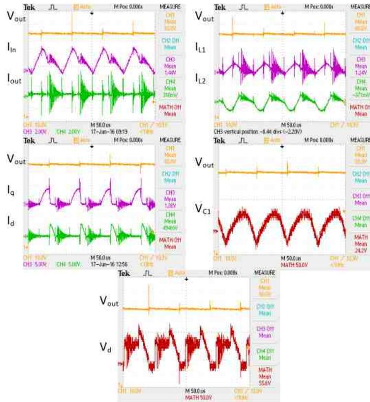
Fig. 4.4. Output Voltage  $V_o$ , Source Current  $I_g$ , Output Current  $I_o$ , Inductors Current  $I_{L1}$  &  $I_{L2}$ , Diode Current  $I_d$ , Transistor Current  $I_q$ , Capacitor  $C_1$  Voltage  $V_{C1}$ , and Diode Voltage  $V_d$  for positive boost mode (60V).
