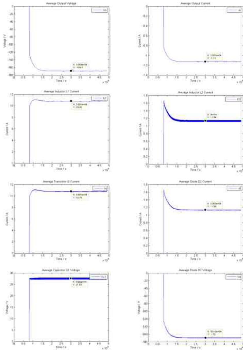
Fig. 2.14. Output Voltage  $V_o$ , Output Current  $I_o$ , Inductors Current  $I_{L1}$  &  $I_{L2}$ , Diode Current  $I_d$ , Transistor Current  $I_q$ , Capacitor  $C_1$  Voltage  $V_{C1}$ , and Diode Voltage  $V_d$  for positive boost mode. (Duty cycle=83.3%,  $V_o=-169.5\text{V}$ ,  $I_o=-1.13\text{A}$ ,  $I_{L1}=10.81\text{A}$ ,  $I_{L2}=1.134\text{A}$ ,  $I_q=10.79\text{A}$ ,  $I_d=1.136\text{A}$ ,  $V_{C1}=27.59\text{V}$ ,  $V_D=-170\text{V}$ )
