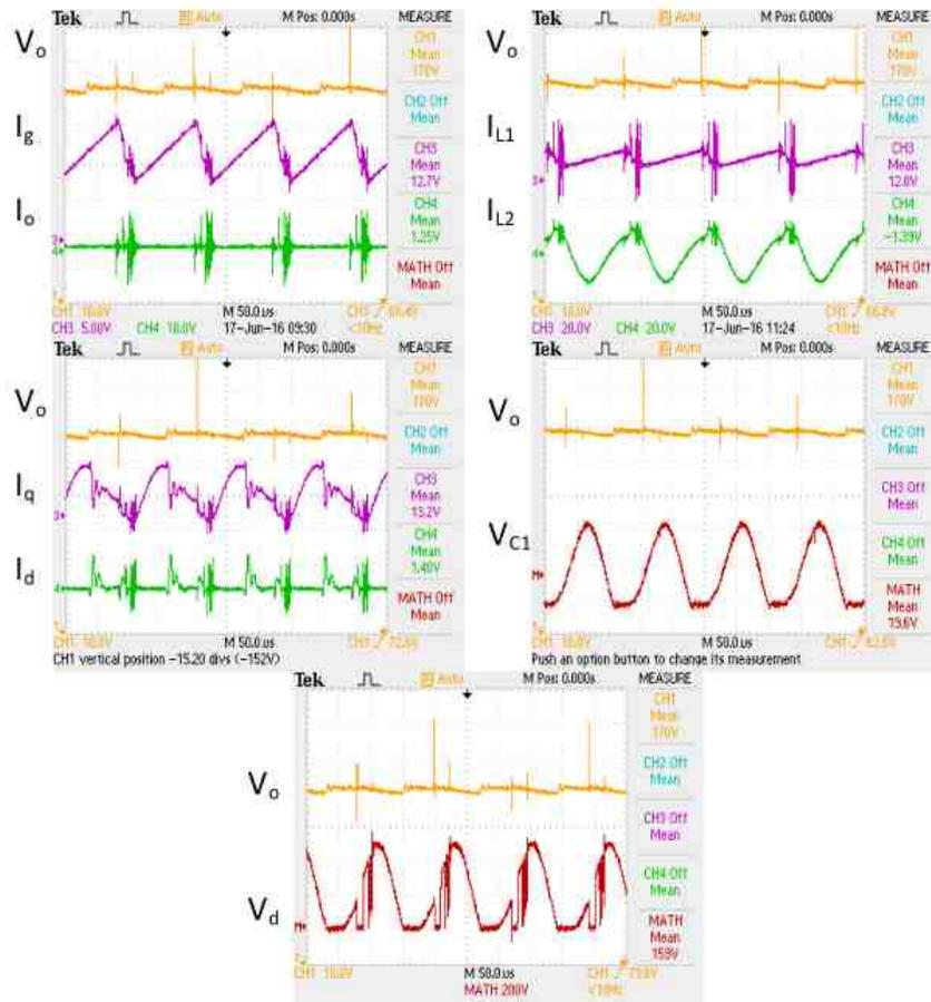
Fig. 4.3. Output Voltage  $V_o$ , Source Current  $I_g$ , Output Current  $I_o$ , Inductors Current  $I_{L1}$  &  $I_{L2}$ , Diode Current  $I_d$ , Transistor Current  $I_q$ , Capacitor  $C_1$  Voltage  $V_{C1}$ , and Diode Voltage  $V_d$  for positive boost mode (170V).
