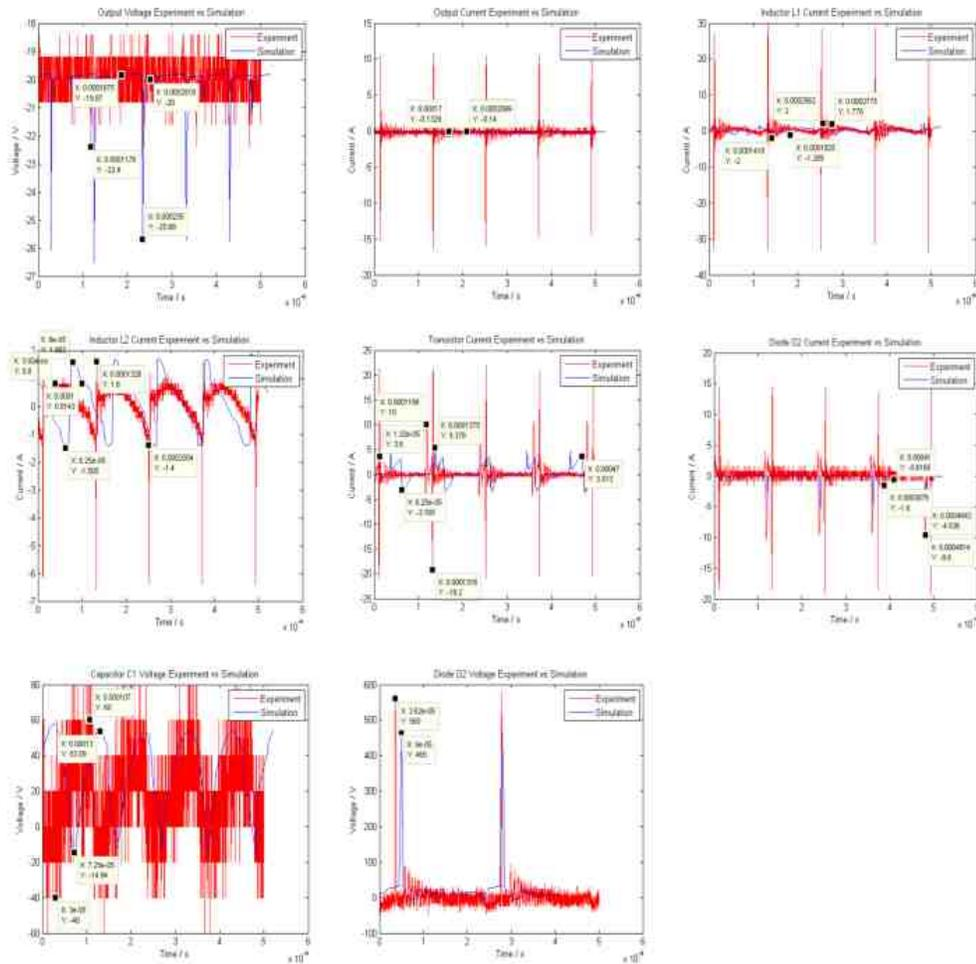
Fig. 4.14. Comparison of Output Voltage  $V_o$ , Source Current  $I_g$ , Output Current  $I_o$ , Inductors Current  $I_{L1}$  &  $I_{L2}$ , Diode Current  $I_d$ , Transistor Current  $I_q$ , Capacitor  $C_1$  Voltage  $V_{C1}$ , and Diode Voltage  $V_d$  for negative buck mode.
