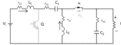
Fig. 2.2. Positive mode I,  $Q$  and  $D_1$  are synchronized,  $Q$ : OFF,  $D_2$ : ON.
