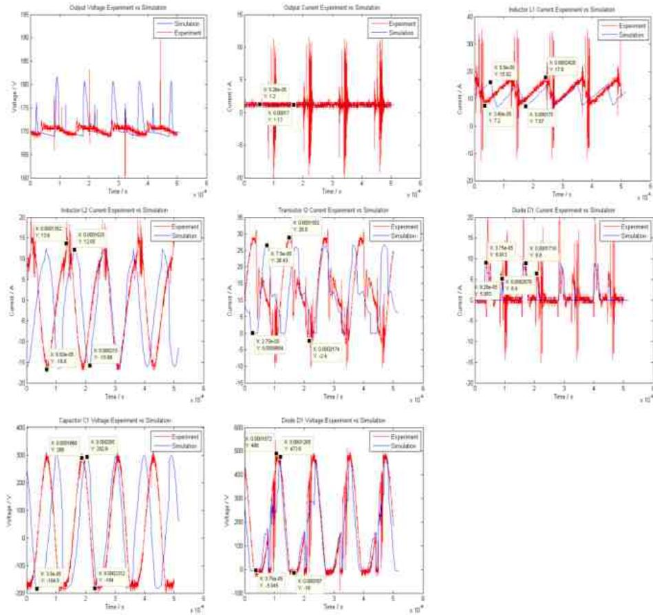
Fig. 4.9. Comparison of Output Voltage  $V_o$ , Source Current  $I_g$ , Output Current  $I_o$ , Inductors Current  $I_{L1}$  &  $I_{L2}$ , Diode Current  $I_d$ , Transistor Current  $I_q$ , Capacitor  $C_1$  Voltage  $V_{C1}$ , and Diode Voltage  $V_d$  for positive boost mode (170V).
