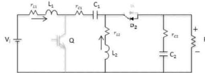
Fig. 2.4. Negative mode I,  $Q$  and  $D_1$  are synchronized,  $Q$ : Off,  $D_2$ : ON.
