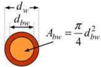
Fig. 4.2. Dimensions of magnet wire
