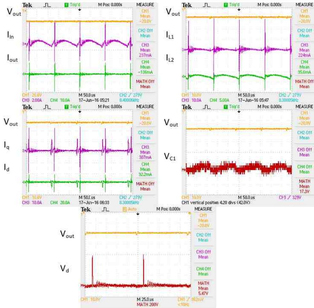
Fig. 4.8. Output Voltage  $V_o$ , Source Current  $I_g$ , Output Current  $I_o$ , Inductors Current  $I_{L1}$  &  $I_{L2}$ , Diode Current  $I_d$ , Transistor Current  $I_q$ , Capacitor  $C_1$  Voltage  $V_{C1}$ , and Diode Voltage  $V_d$  for positive buck mode.
