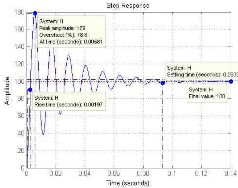
Fig. 3.13. Step Response for Negative Output Voltage
