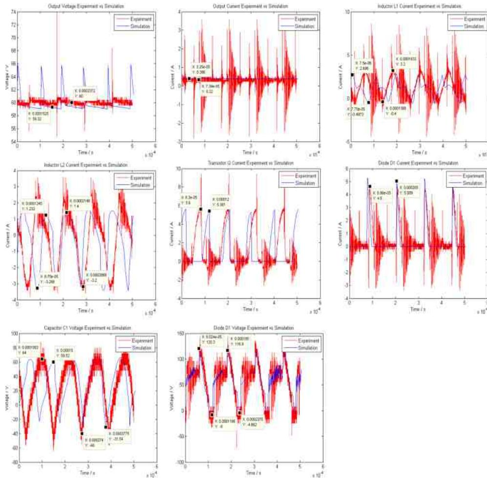
Fig. 4.10. Comparison of Output Voltage  $V_o$ , Source Current  $I_g$ , Output Current  $I_o$ , Inductors Current  $I_{L1}$  &  $I_{L2}$ , Diode Current  $I_d$ , Transistor Current  $I_q$ , Capacitor  $C_1$  Voltage  $V_{C1}$ , and Diode Voltage  $V_d$  for positive boost mode (60V).
