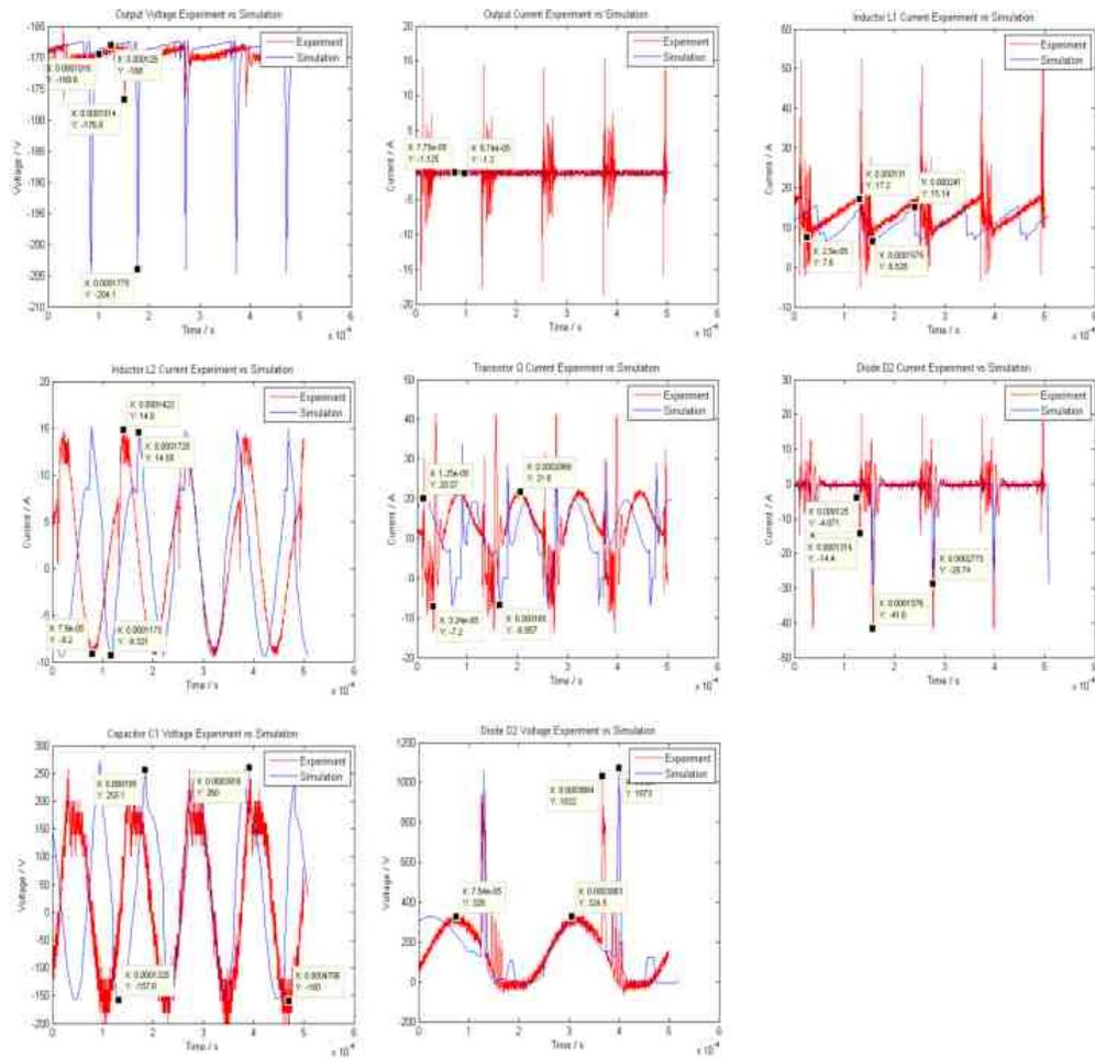
Fig. 4.12. Comparison of Output Voltage  $V_o$ , Source Current  $I_g$ , Output Current  $I_o$ , Inductors Current  $I_{L1}$  &  $I_{L2}$ , Diode Current  $I_d$ , Transistor Current  $I_q$ , Capacitor  $C_1$  Voltage  $V_{C1}$ , and Diode Voltage  $V_d$  for negative boost mode (-170V).
