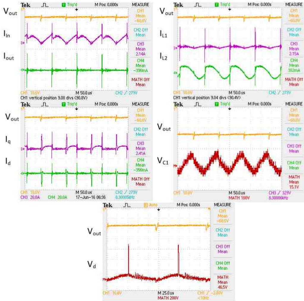
Fig. 4.7. Output Voltage  $V_o$ , Source Current  $I_g$ , Output Current  $I_o$ , Inductors Current  $I_{L1}$  &  $I_{L2}$ , Diode Current  $I_d$ , Transistor Current  $I_q$ , Capacitor  $C_1$  Voltage  $V_{C1}$ , and Diode Voltage  $V_d$  for positive boost mode (-60V).
