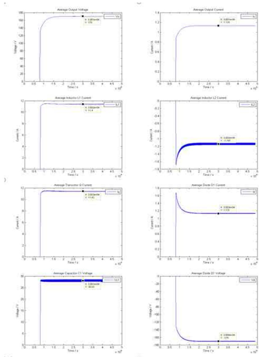
Fig. 2.11. Output Voltage  $V_o$ , Output Current  $I_o$ , Inductors Current  $I_{L1}$  &  $I_{L2}$ , Diode Current  $I_d$ , Transistor Current  $I_q$ , Capacitor  $C_1$  Voltage  $V_{C1}$ , and Diode Voltage  $V_d$  for positive boost mode. (Duty cycle=79.5%,  $V_o=170$ V,  $I_o=1.133$ A,  $I_{L1}=11.4$ A,  $I_{L2}=-1.141$ A,  $I_q=11.42$ A,  $I_d=1.131$ A,  $V_{C1}=28.03$ V,  $V_D=170$ )
