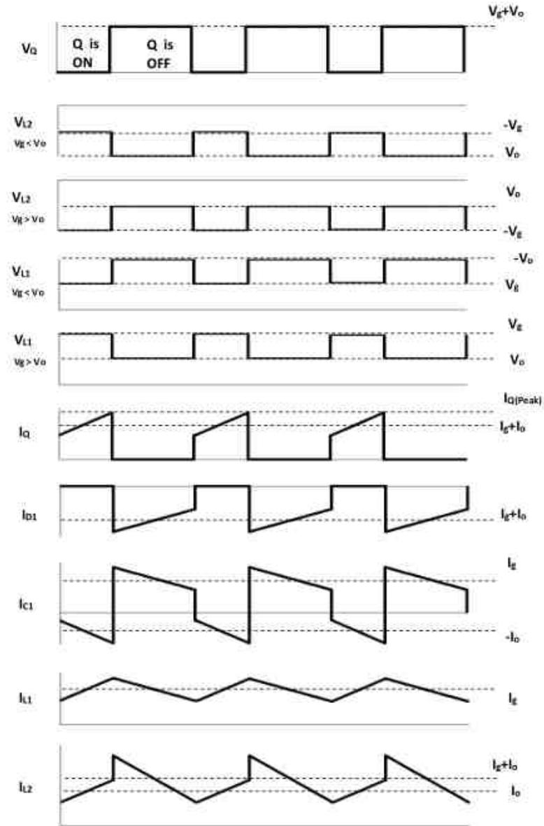
Fig. 2.7. Voltages and currents of the components in the converter under the positive mode
