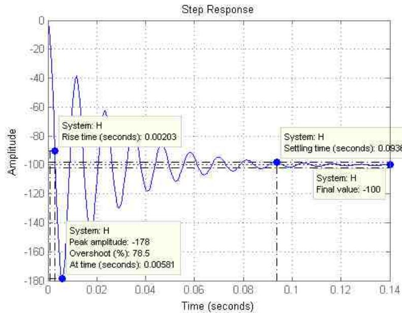
Fig. 3.14. Step Response for Positive Output Voltage
