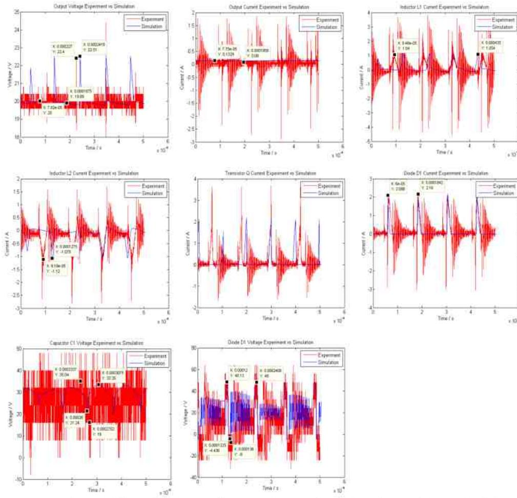
Fig. 4.11. Comparison of Output Voltage  $V_o$ , Source Current  $I_g$ , Output Current  $I_o$ , Inductors Current  $I_{L1}$  &  $I_{L2}$ , Diode Current  $I_d$ , Transistor Current  $I_q$ , Capacitor  $C_1$  Voltage  $V_{C1}$ , and Diode Voltage  $V_d$  for positive buck mode.
