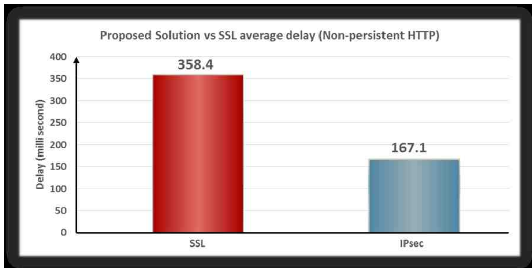
Fig. 5.9. SSL vs Proposed Solution Average Delay (non-persistent HTTP)
