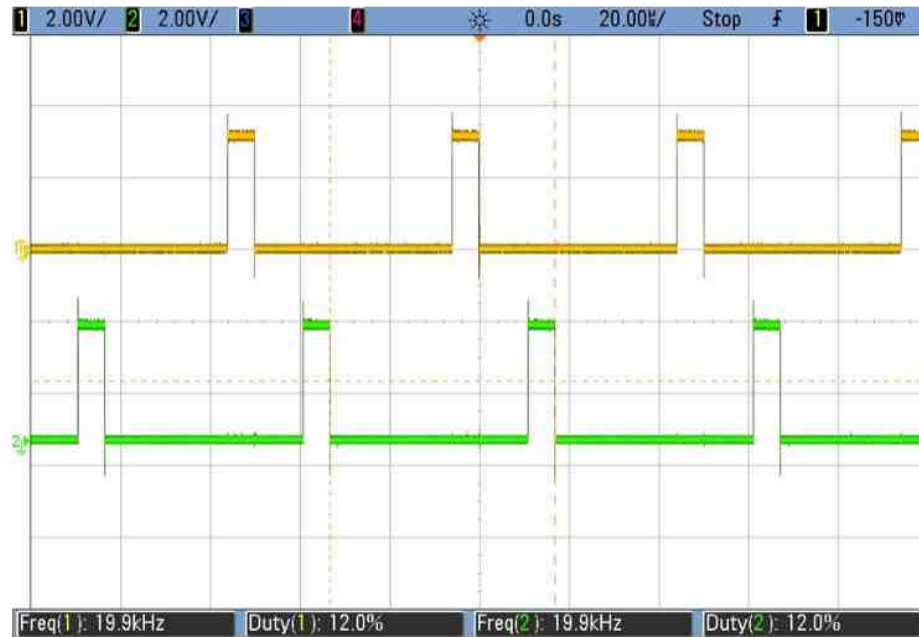
Fig. 5.3. Wireless Link Distance of 1 foot, ma = 0.12 .
