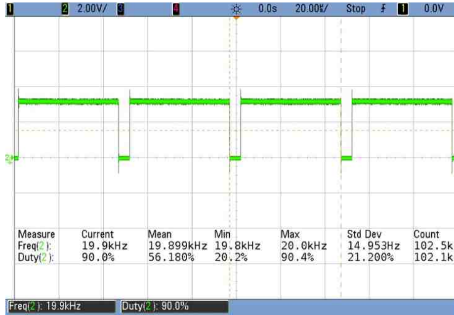
Fig. 5.8. Wireless Link Distance of 18 feet, m_a = 0.9 .
