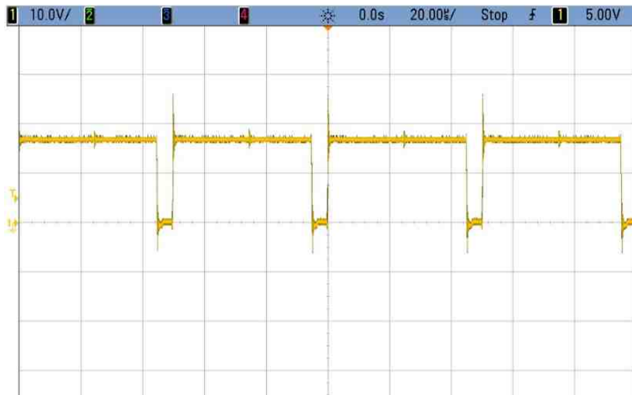
Fig. 5.18. PWM for m_a = 0.9 , DC Motor Application.
