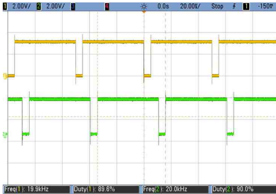
Fig. 5.5. Wireless Link Distance of 1 foot, m_a = 0.9 .
