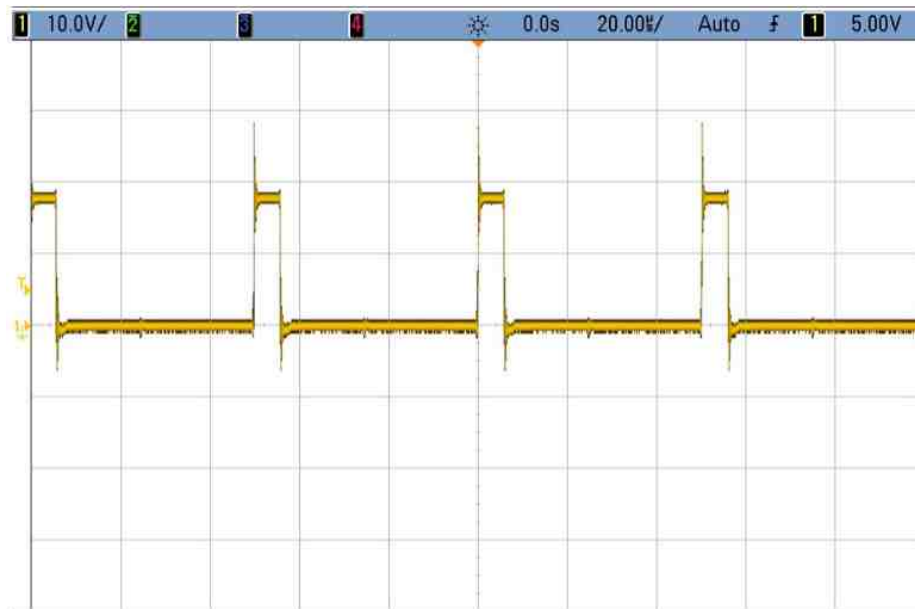
Fig. 5.16. PWM for m_a = 0.12 , DC Motor Application.
