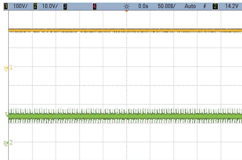
Fig. 4.19. Experimental results showing the boost converter: the first signal (yellow) is the boosted voltage, and the second (green) is the input.
