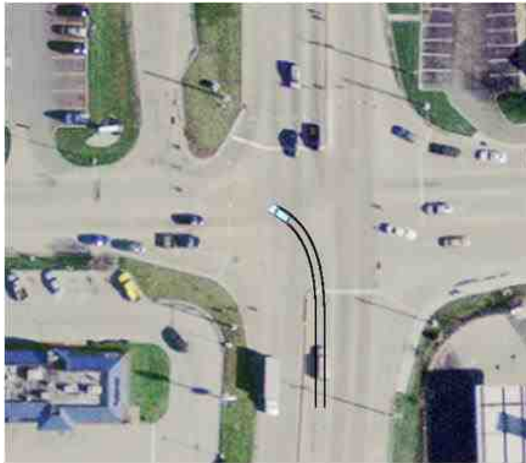
Fig. 6.6. Escape trajectory for scaled steering-angle data
