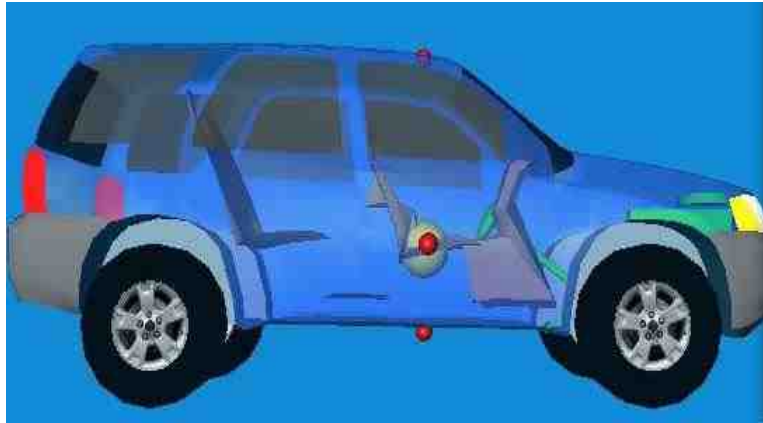
(a) Geometric profile of the Ford Escape: The circle near the center of the vehicle indicates the center of gravity
