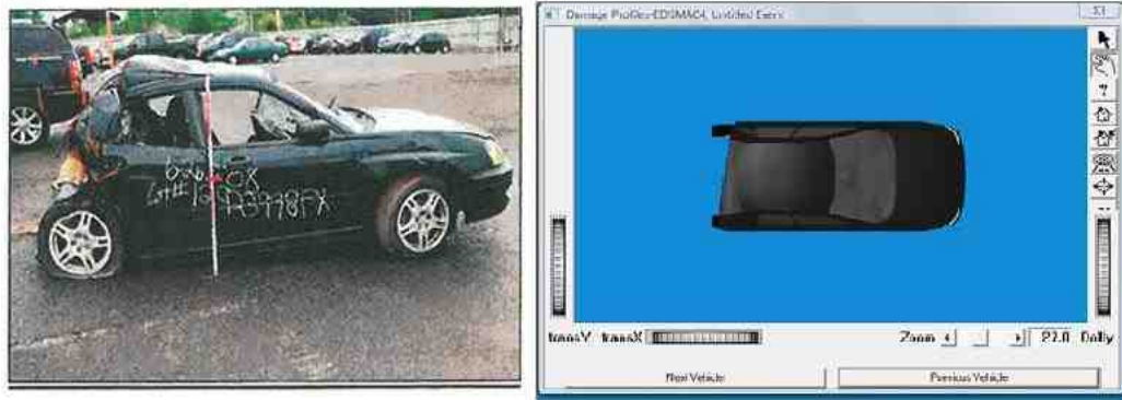
(a) Subaru real life and simulated damage profile
