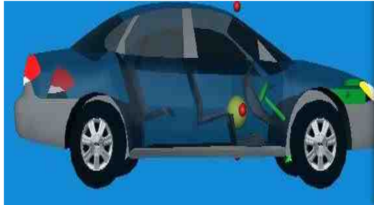
(a) Geometric profile of the Ford Taurus: The circle near the center of the vehicle indicates the center of gravity
