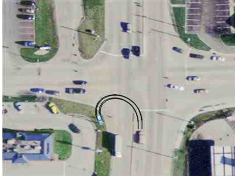
Fig. 6.3. Escape trajectory using original steering angle profile
