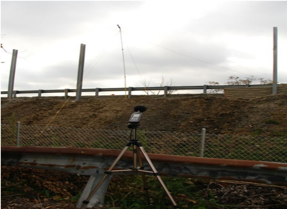
Fig. 3.5. Picture of SLM setup. Notice the reference and the local SLM
