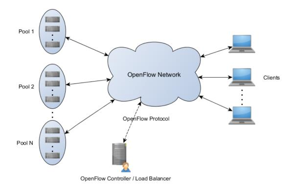
Fig. 3.1. Round robin load balancing with OpenFlow
