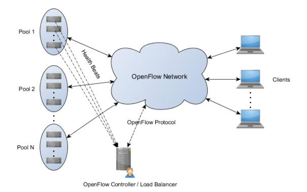
Fig. 3.2. Load based load balancing with OpenFlow
