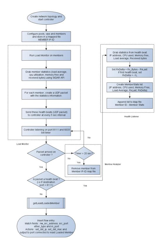
Fig. 3.3. Flowchart explaining various steps in load based algorithm
