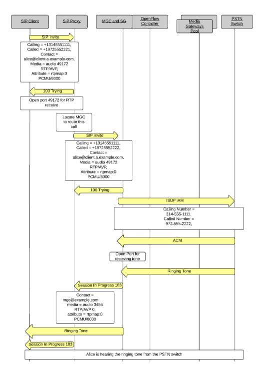
Fig. 5.8. Event diagram for SIP-PSTN architecture integrated with Open-Flow load balancing [Contd..]
