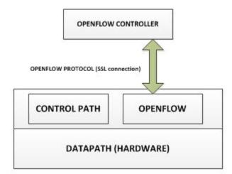
Fig. 1.2. Basic functional diagram of an OpenFlow switch and controller
