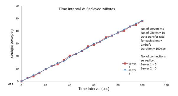
Fig. 4.4. Received load by servers at an instance of time for fixed data transfer rate (round robin algorithm)
