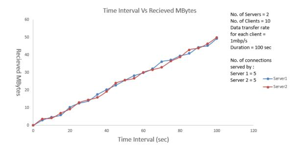
Fig. 4.6. Received load by servers at an instance of time for fixed data transfer rate (load based algorithm)
