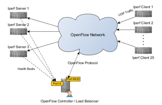
Fig. 4.3. Experiment setup
