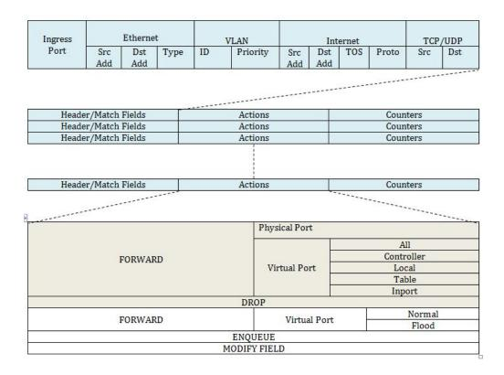
Fig. 1.4. Structure of a flow-entry table
