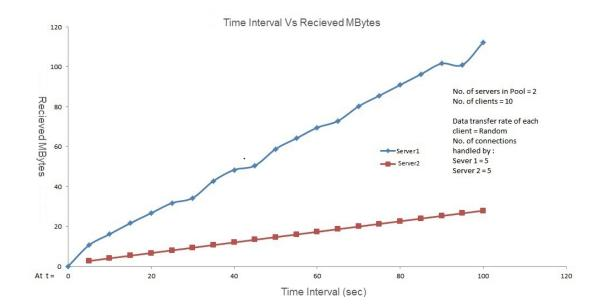
Fig. 4.5. Received load by servers at an instance of time for random data transfer rate (round robin algorithm)
