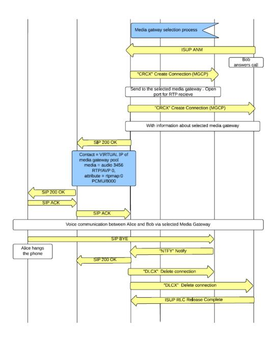
Fig. 5.9. Event diagram for SIP-PSTN architecture integrated with Open-Flow load balancing
