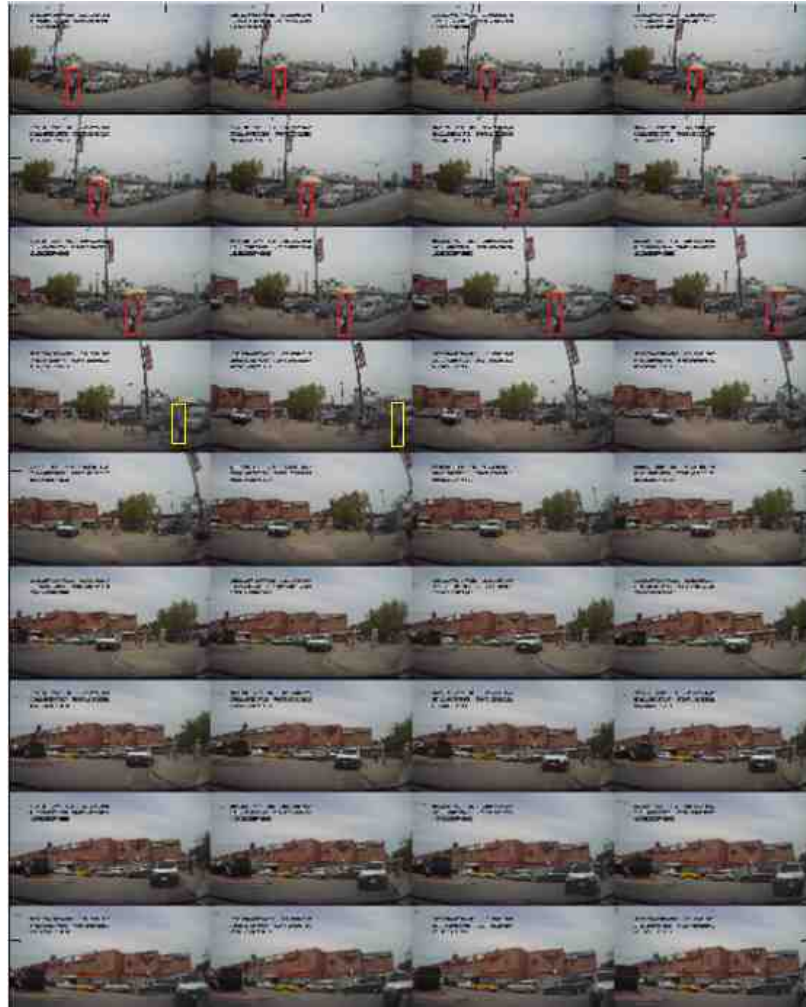
Fig. 5.2. Sample vary good tracking frame sequence (every 4 frames with red boxes as tracked pedestrian location, blue boxes as tracking mistakes and yellow boxes as missed pedestrian)
