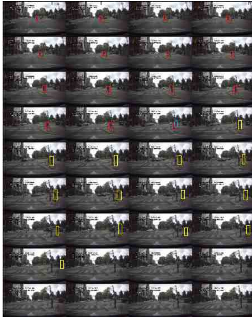
Fig. 5.3. Sample good tracking frame sequence (every 4 frames with red boxes as tracked pedestrian location, blue boxes as tracking mistakes and yellow boxes as missed pedestrian)
