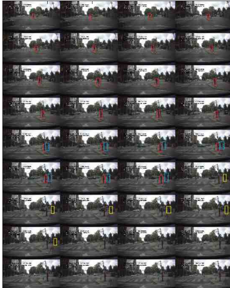
Fig. 5.10. Tracking results by covariance matrix for fair tracking category (every 4 frames with red boxes as tracked pedestrian location, blue boxes as tracking mistakes and yellow boxes as missed pedestrian)
