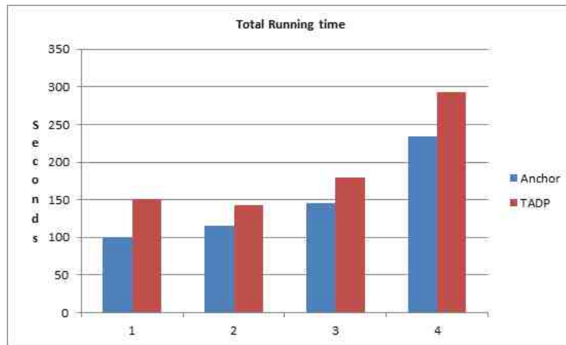
Fig. 4.26: Comparison of the total running time of Bus_cif for different QP values
