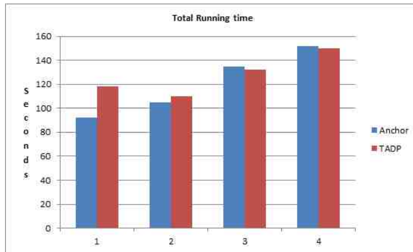
Fig. 4.28: Comparison of the total running time of Mobile_cif for different QP values
