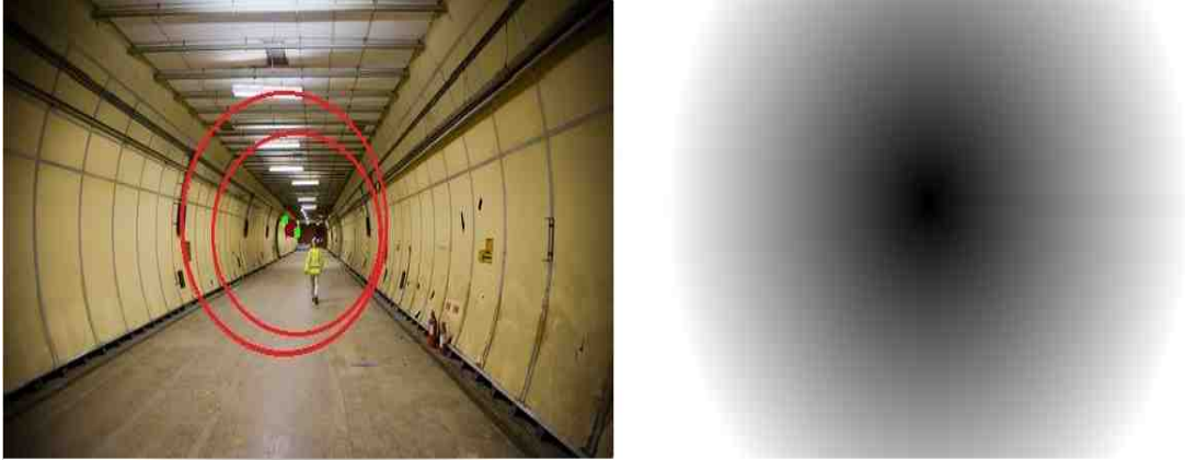
Fig. 2.15. Example of depth gradient generated (right) on tunnel image from circle detection (left)
