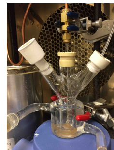
(b) Reaction chamber of MIMS
