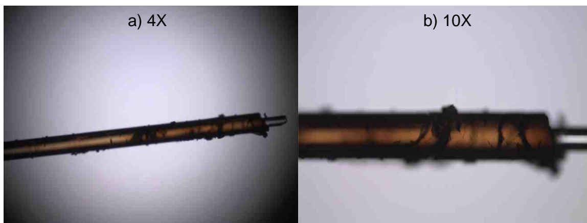
Figure 6-3 Microscopic images of a polyacrylate fiber after ~20 uses of TV-SPME of 120 \mu L chloroform hair extracts. a) image taken at 4X b) image taken at 10X
