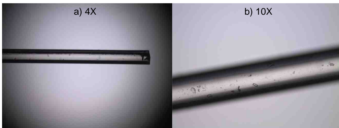
Figure 6-1 Microscopic images of a polyacrylate fiber prior to conditioning or use. a) image taken at 4X b) image taken at 10X
