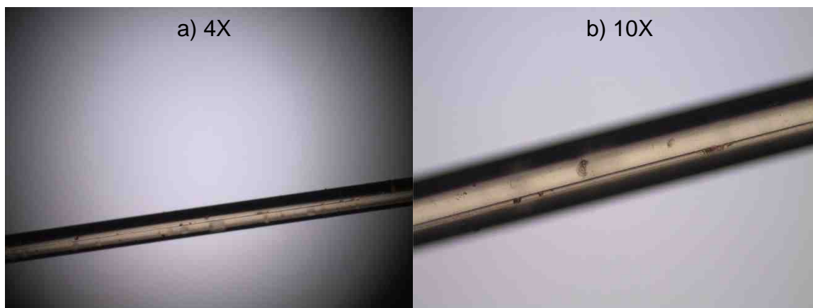
Figure 6-2 Microscopic images of a polyacrylate fiber after conditioning at 280°C for 1 hr. a) image taken at 4X b) image taken at 10X
