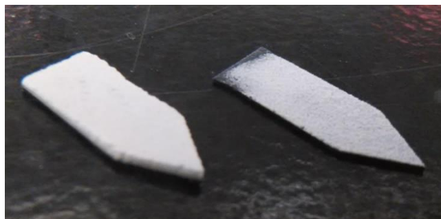
Figure 3.1: TLC Spray Substrates. Cut TLC spray substrates with a thick (left) and thin (right) stationary phase.
