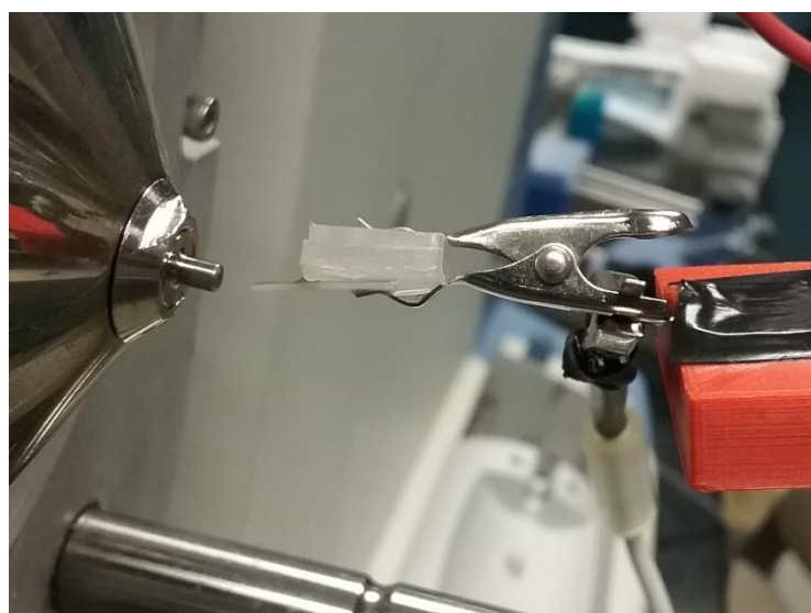
Figure 6.3: Paper Spray Analysis of Cytochrome C. Paper spray MS analysis of cytochrome C using a 3D printed solvent well clipped onto porous polyethylene positioned in front of a mass spec inlet.
