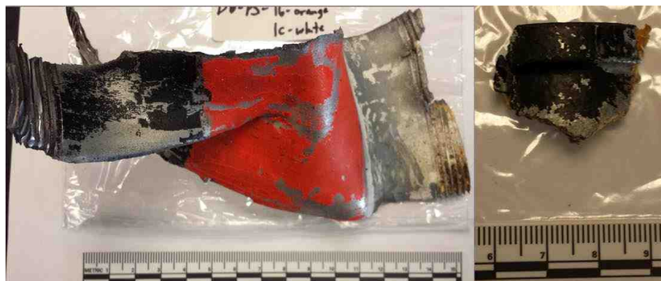
Figure 6-2 Fragments used to calculate V_{50} velocities.
