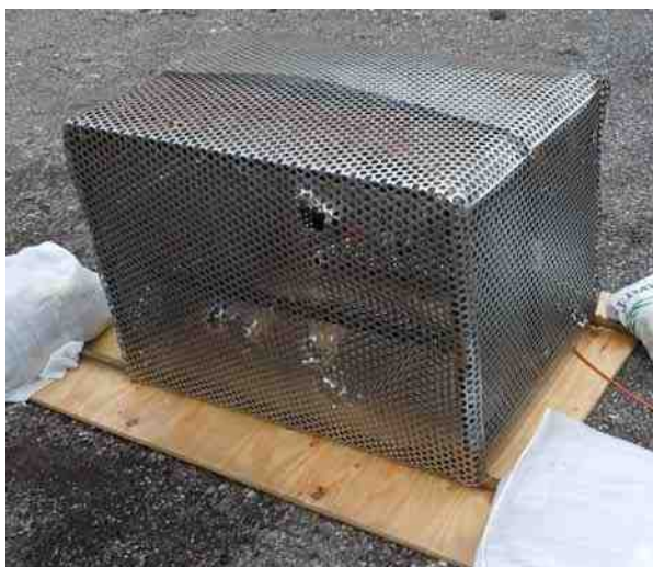
Figure 6-3 Containment structure after multiple initiations of steel devices.
