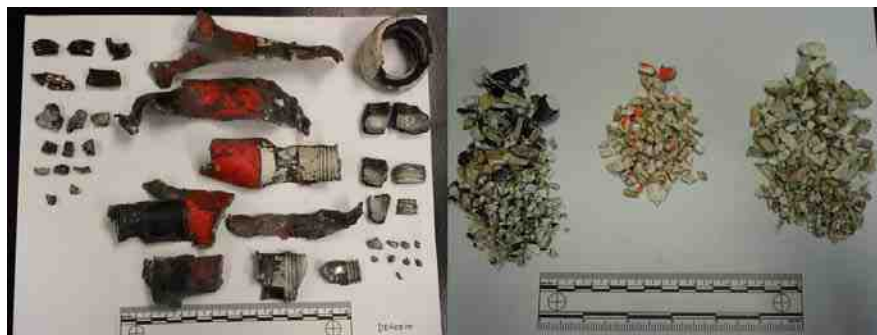
Figure 4-3 Reconstruction of both device types (L: steel; R: PVC).
