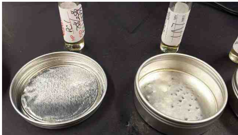
Figure 6-6 Post evaporation of commercially available track adhesives (Left: poly (ethyl ether) based; right: fatty acid based).
