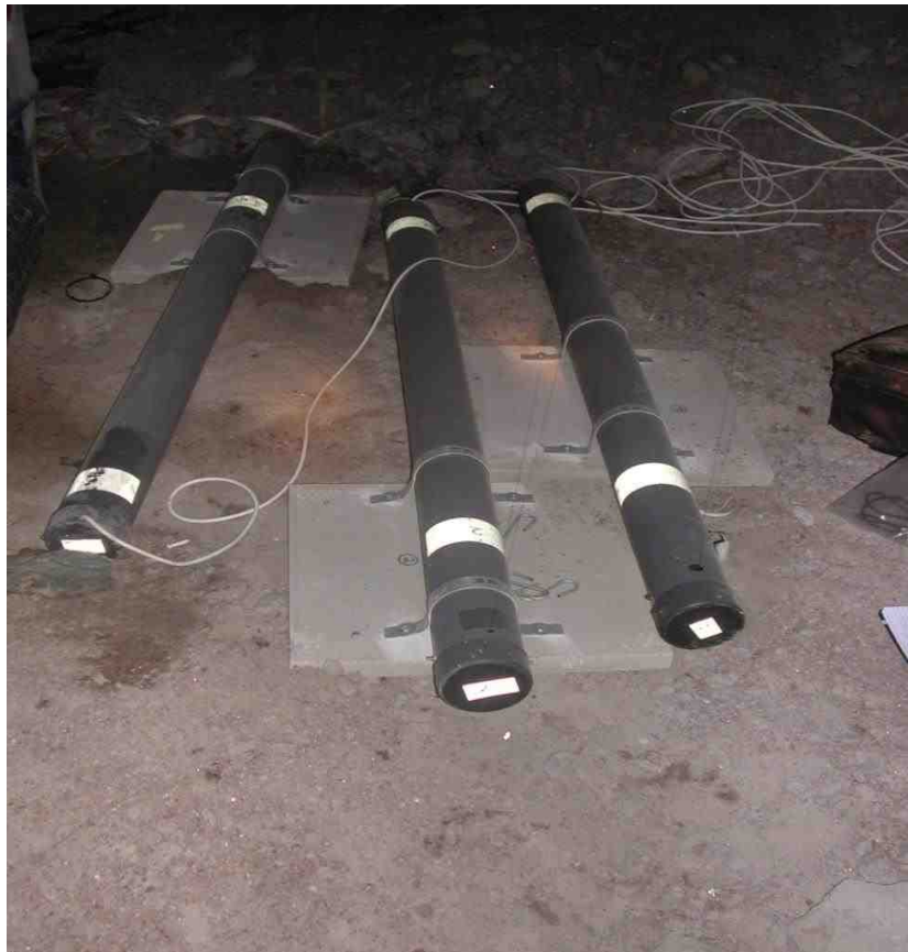
Plate 4.4 Closuremeters installed at stub of an ongoing mined panel
