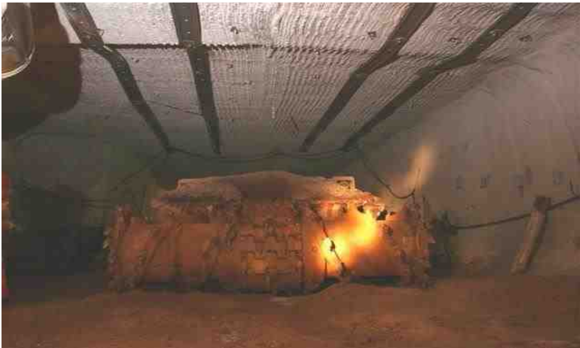
Plate 3.1 A continuous miner at a working salt face at Boulby mine (source Boulby, 2009)
