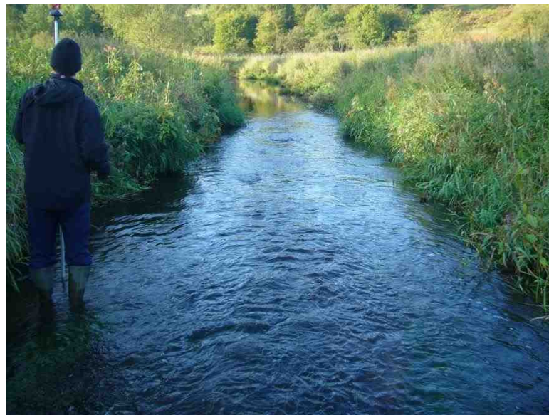
Figure 3.2: Photo showing the surface expressions of submerged vegetation canopies. Flow is from bottom to top. The river is approximately 5m wide and 0.3m deep. The water surface deviations from the mean are estimated as less than 10% of the flow depth.
