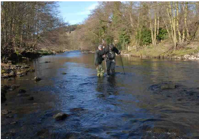
Figure 4.5: Kick sampling for macroinvertebrates. Whilst two people are shown here, often the samples taken were carried out alone. The nature of the streams made this relatively safe.
