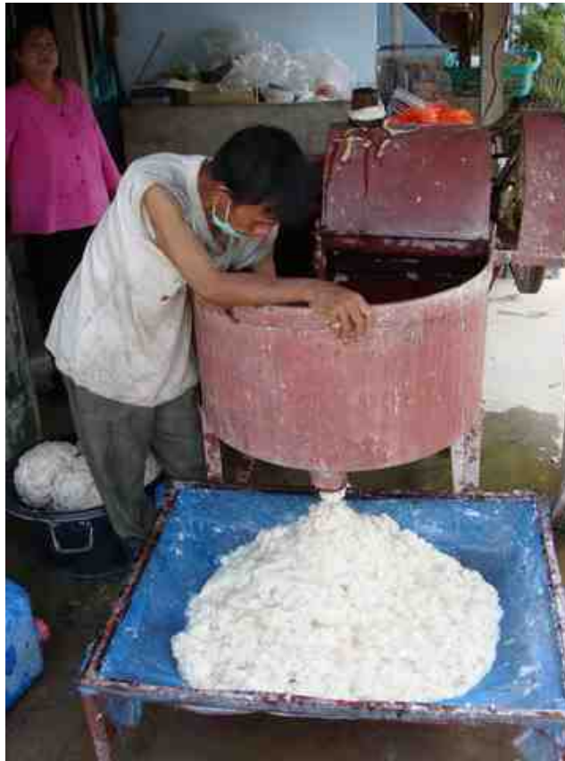
Picture 5.6 Shredding Machine to Make Smaller Fibres
