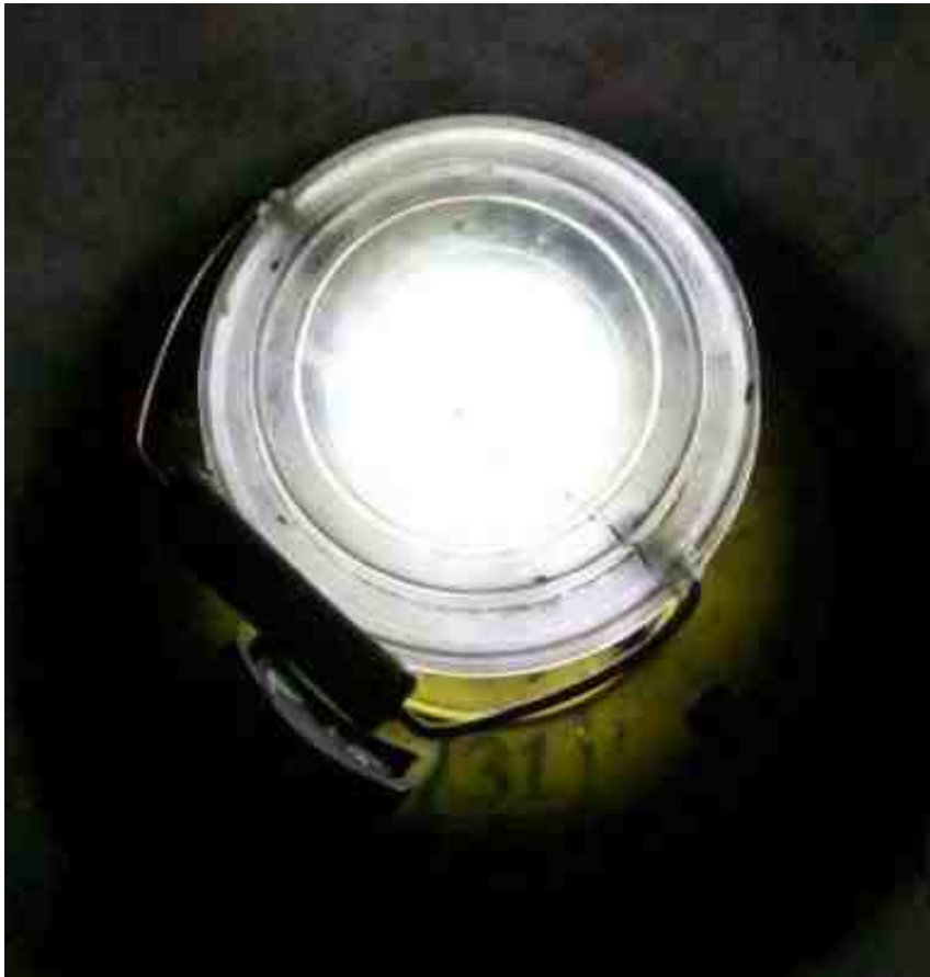
Figure 5-9: Solar lantern with an open switch panel.
