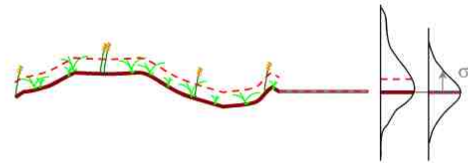
Figure 1.4 Systematic upward shift \sigma in laser measurements over low vegetation. The dashed line illustrates the expectancy of LiDAR-derived height values. Source: Pfeifer et al. (2004).
