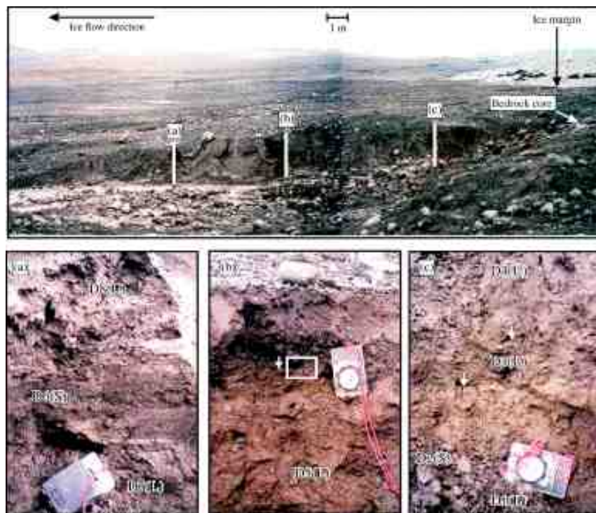
Figure 2.4. Photograph of a stream-cut drumlin exposure, Iceland (top image) with 3 stratigraphic logs (a – c) (Fuller and Murray, 2002). An upper and lower till were identified with clay bands and sand lenses also present.
