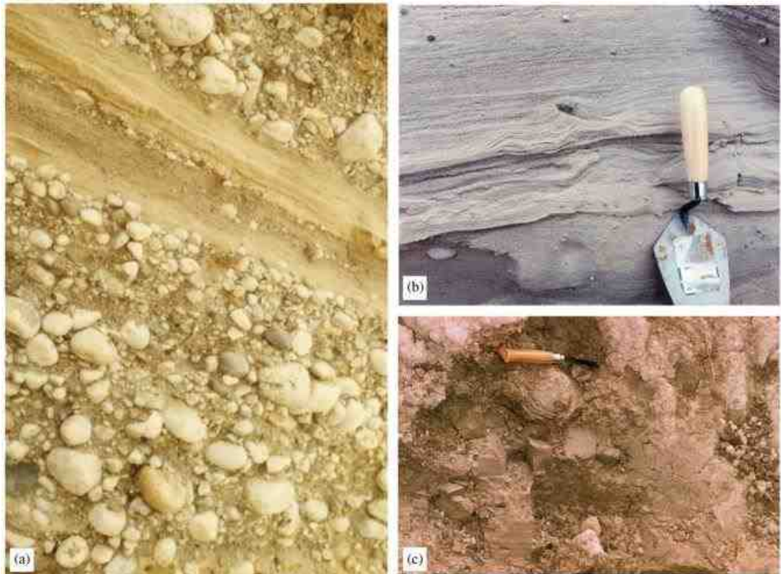
Figure 2.6. Steeply dipping, interbedded sand and gravel (a), medium to fine sands (b) and a reddish brown till reported within the drumlin illustrated in Figure 2.5 (Menzies and Brand, 2007).
