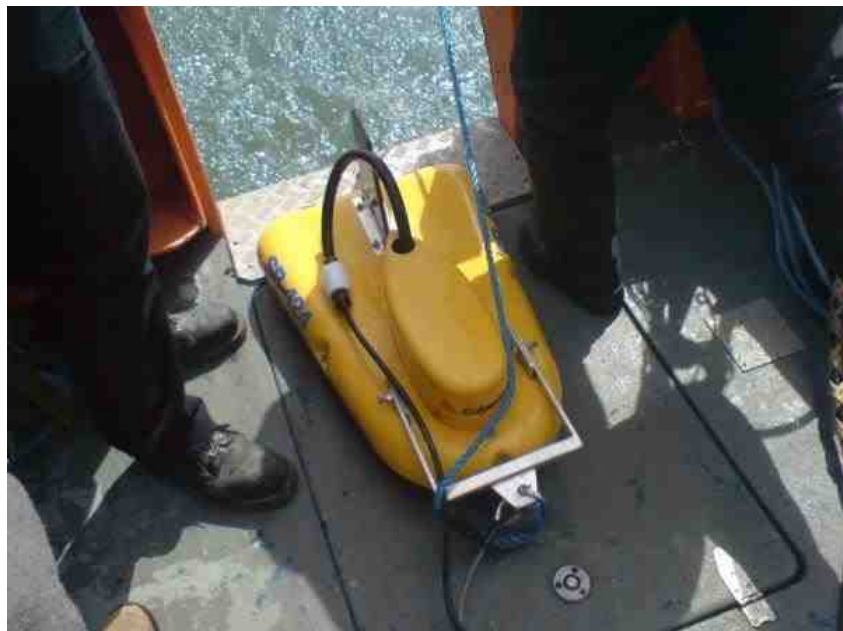
Figure 4.1. The SB-424 Sub-bottom profiling ‘towfish’ that is pulled through the water column behind the towing vessel.
