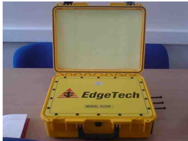
Figure 4.4. 565P Topside processing unit which records all data collected from the attached towfish and transfers data to the laptop unit for visual analysis.
